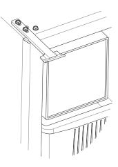
13. Place the door latch assembly on opposite side of unit. Be sure to tighten all three screws securely.
