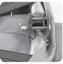
Place (1) cap nut (J) onto end of bolt.
