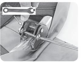
Hold the cap nut using the wrench (M). Tighten using the Phillips screwdriver (N). Repeat these steps to secure hinge on opposite side.
