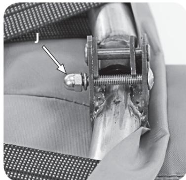
Place (1) cap nut (J) onto end of bolt.
