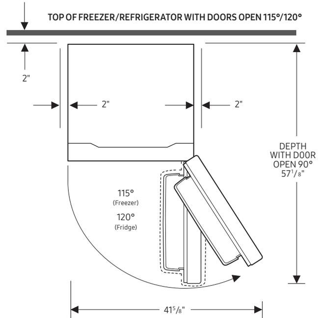
NOTE: Please allow 3<sup>3</sup>/<sub>4</sub>" of clearance when installing along a wall.
