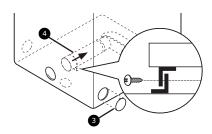
3 Preassemble a 4" (10.2 cm) elbow 5 to the next 4" (10.2 cm) duct section, and secure all joints with duct tape. Be sure that the male end of the elbow faces AWAY from the dryer. Insert the elbow/duct assembly through the side opening and press it onto the adapter duct. Secure it in place with duct tape. Be sure that the male end of the duct protrudes 1.5" (3.8 cm) to connect the remaining ductwork. Attach the cover plate 6 to the back of the dryer with the included screw.
