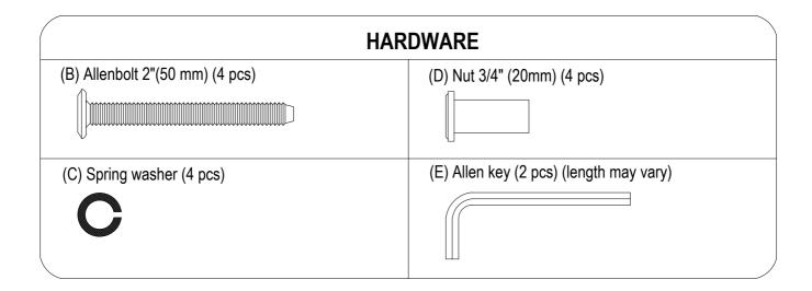
Do not fully tighten all bolts until all parts are in place. (please add an extra 1/2 revolution to the bolts when using spring washer after tightening)
