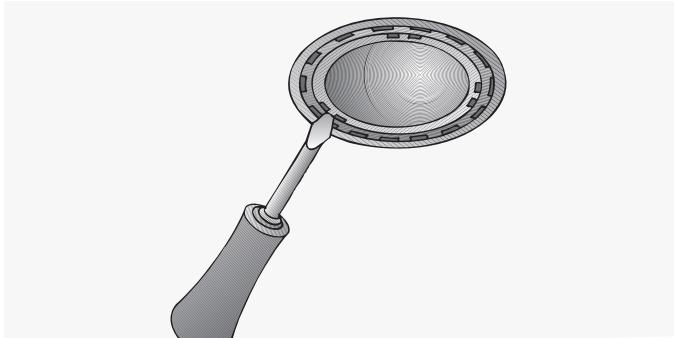
3. Replace the halogen light bulb (conventional halogen bulb, 12 volts, 20 watts max., G4 bulb socket).
