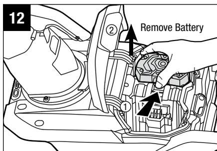
**NOTICE:** Make sure that the latch on the snow blower snaps into place and that the battery pack(s) are secured to the unit before starting operation.
