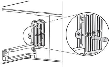
**3** Press on the hooks at the air filter and then take it out.
