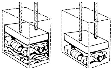
Load bulky trash, bottles, and cans in the center of the drawer. Bottles or cans not placed in the center may become caught between the ram and the drawer. The Drawer Monitor Switch then senses a "misload" and causes the ram to return to the "up" position without compacting.
