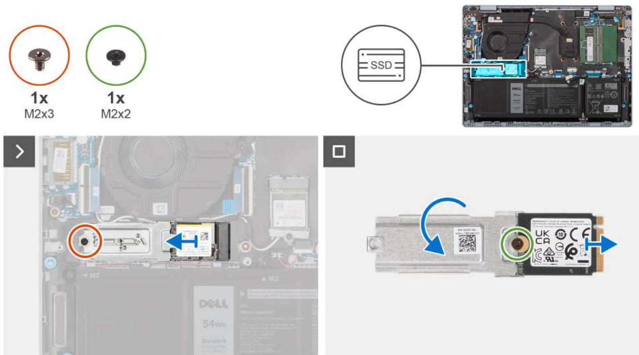
Figure 23. Removing the solid state drive
