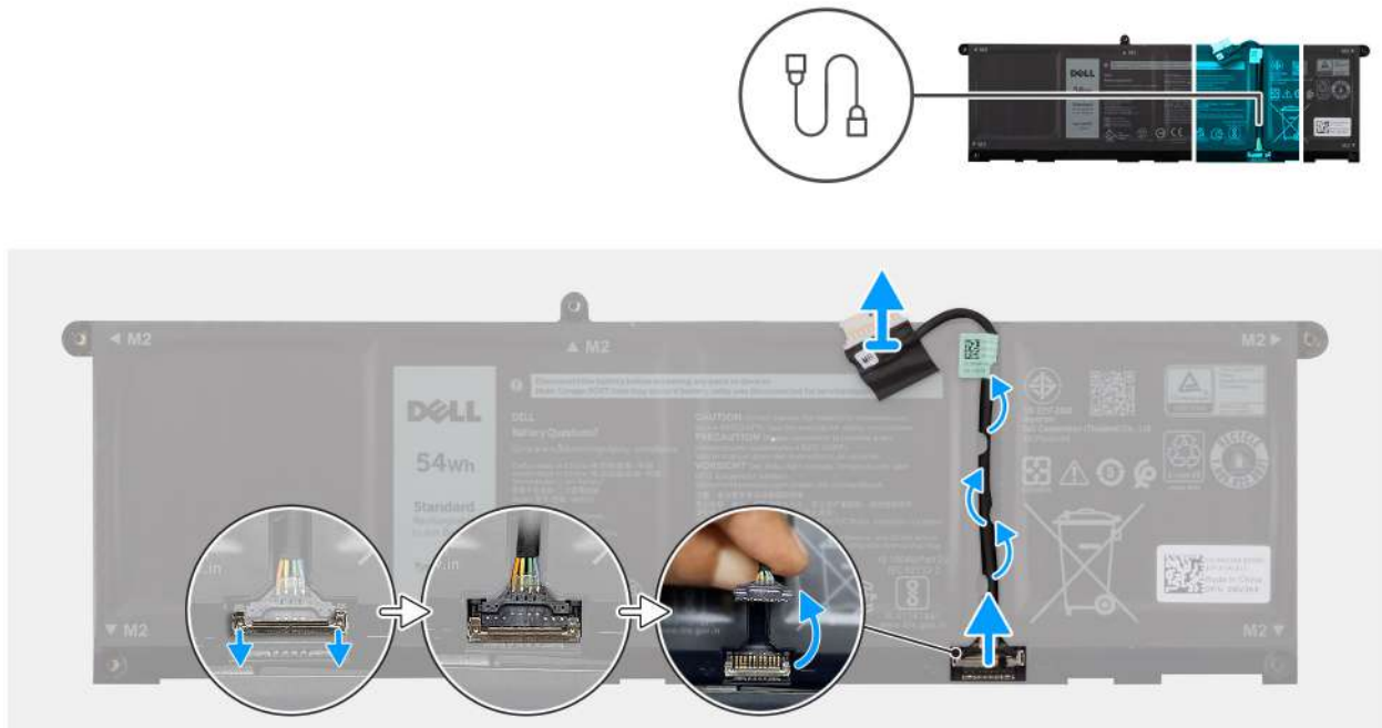
Figure 19. Disconnecting the battery cable
