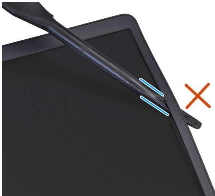
Figure 60. Removing the display bezel
