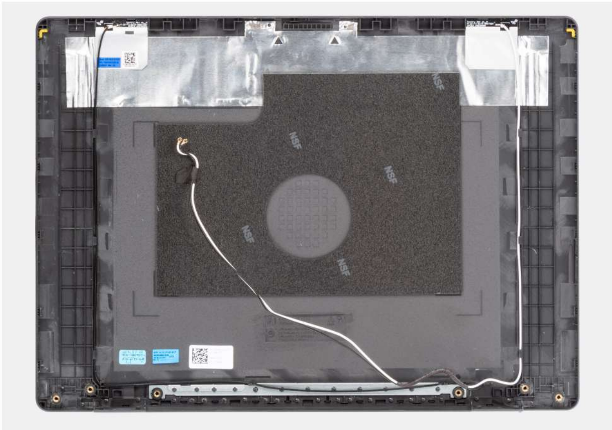
Figure 76. Display back-cover and antenna assembly
