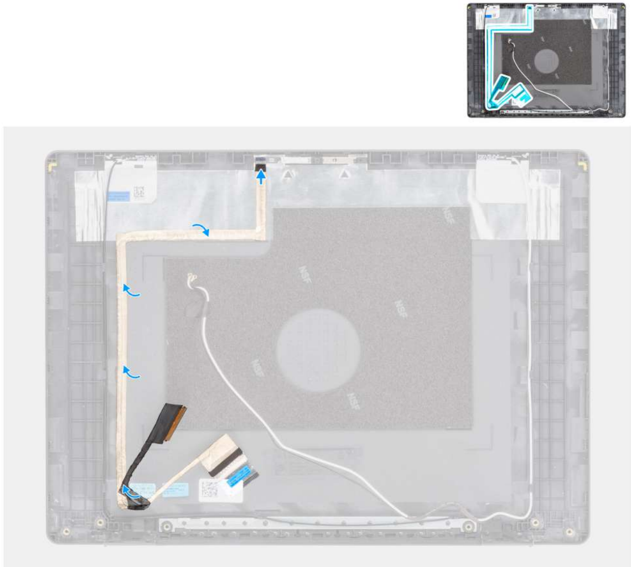
Figure 73. Installing the display cable
