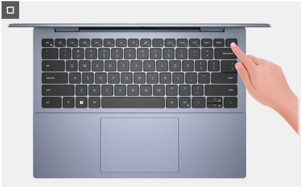
Figure 11. Pressing the power button to drain flea power
