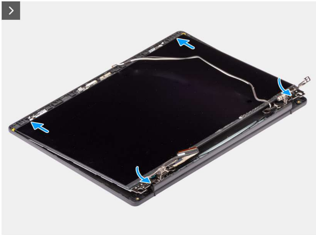
Figure 69. Installing the display panel
