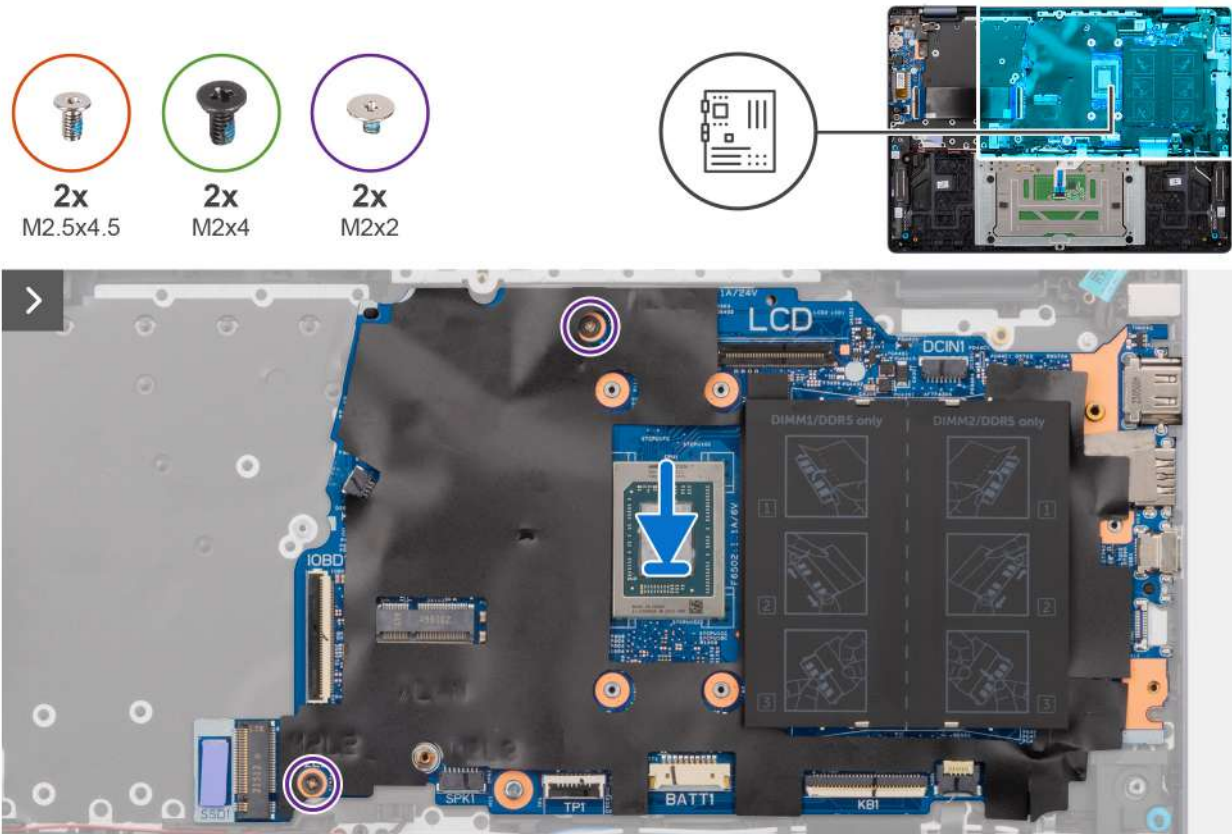
Figure 92. Installing the system board (for computers shipped with an aluminum chassis)
