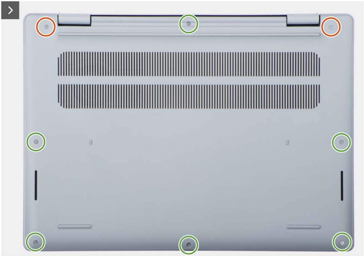
Figure 1. Removing the base cover
