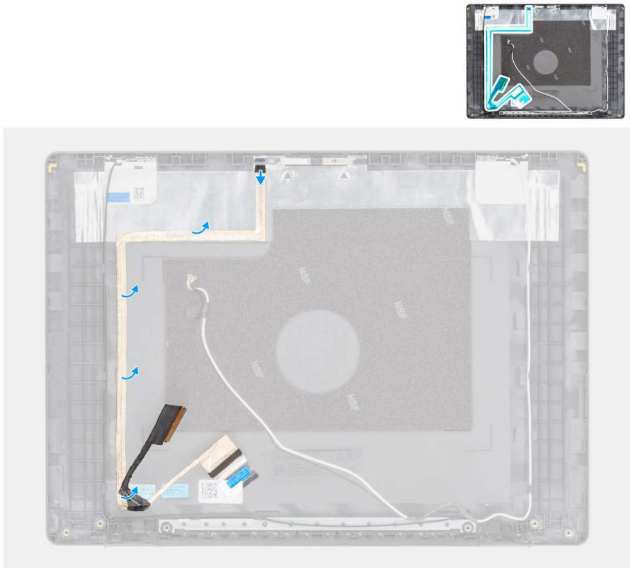
Figure 72. Removing the display cable
