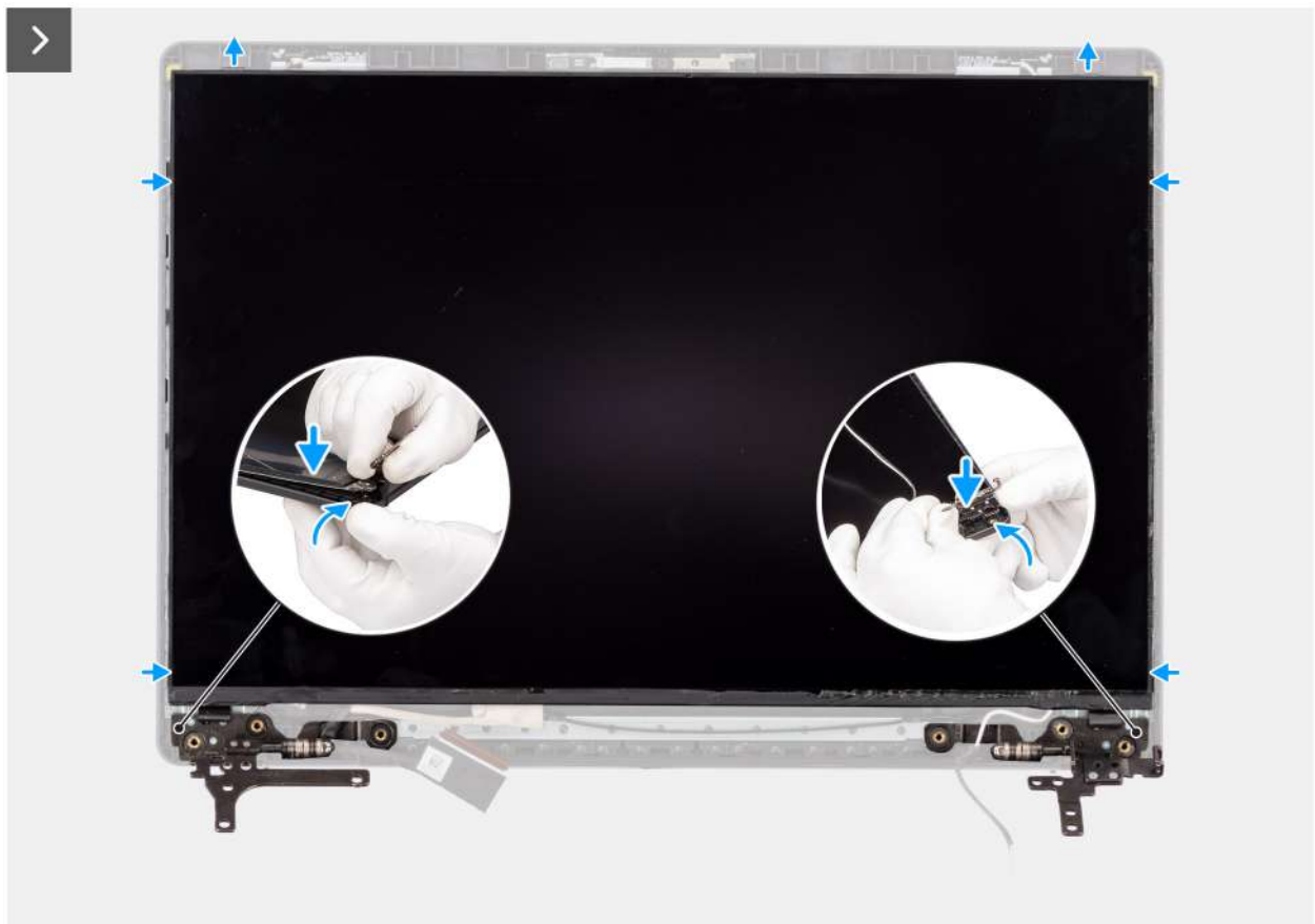
Figure 70. Installing the display panel
