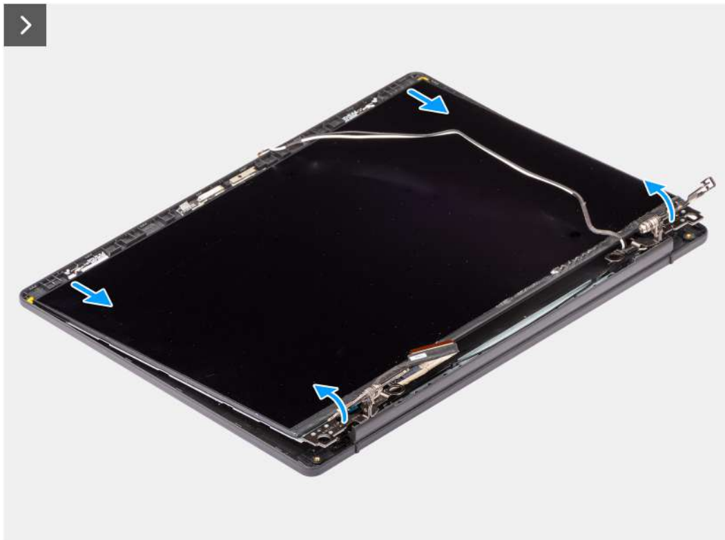
Figure 65. Removing the display panel
