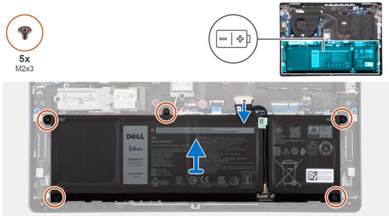
Figure 17. Removing the battery
