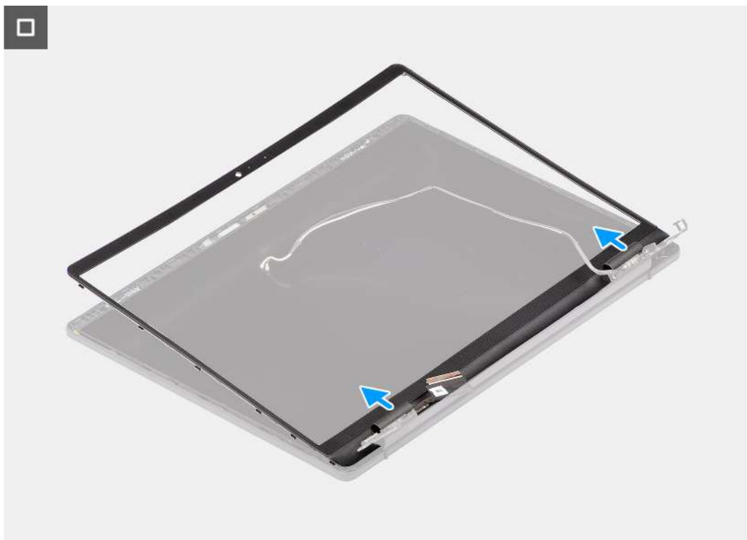
Figure 59. Removing the display bezel
