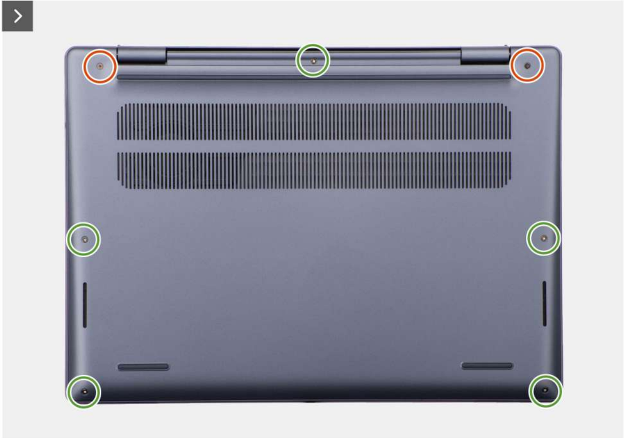
Figure 8. Removing the base cover
