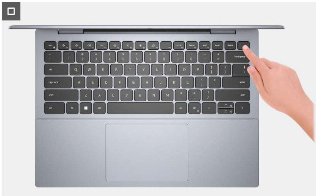
Figure 4. Pressing the power button to drain flea power
