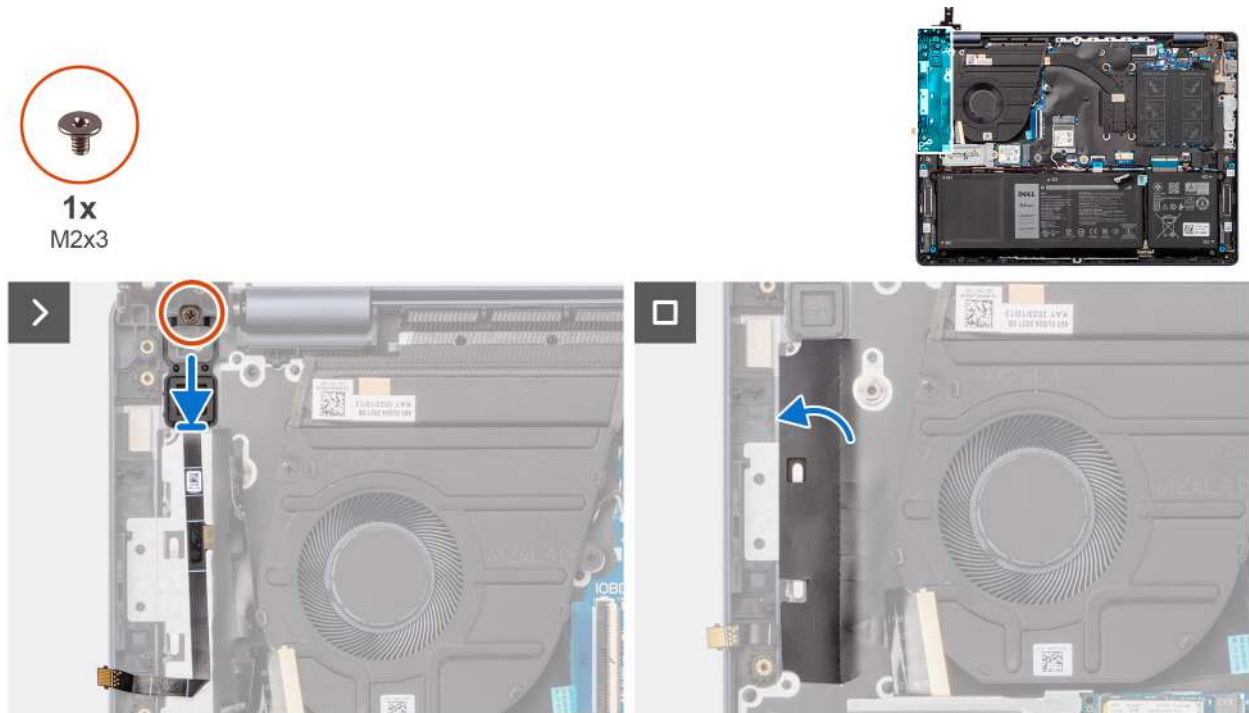
Figure 50. Installing the power button with the optional fingerprint reader
