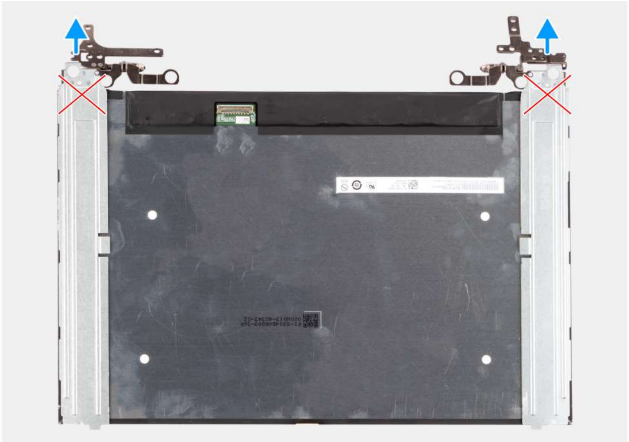
Figure 67. Removing the display panel
