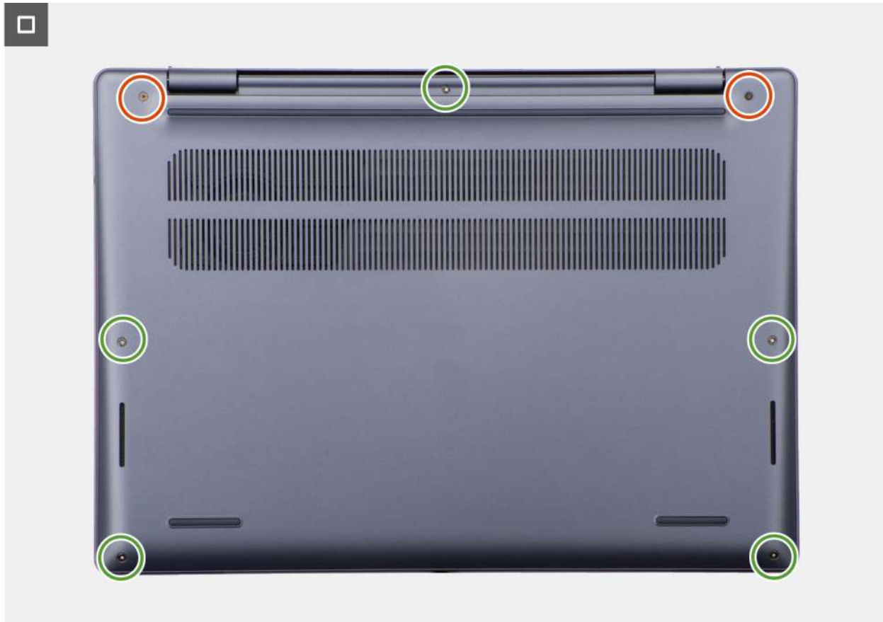
Figure 14. Installing the base cover
