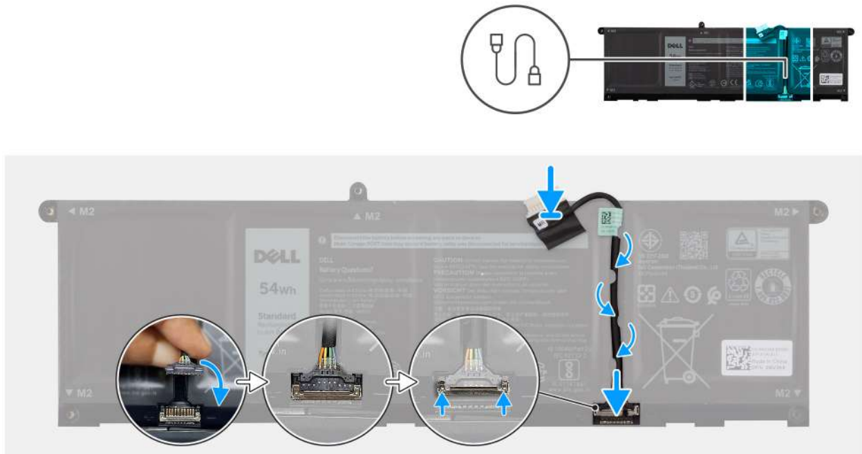
Figure 20. Connecting the battery cable
