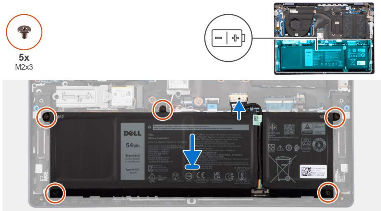
Figure 18. Installing the battery
