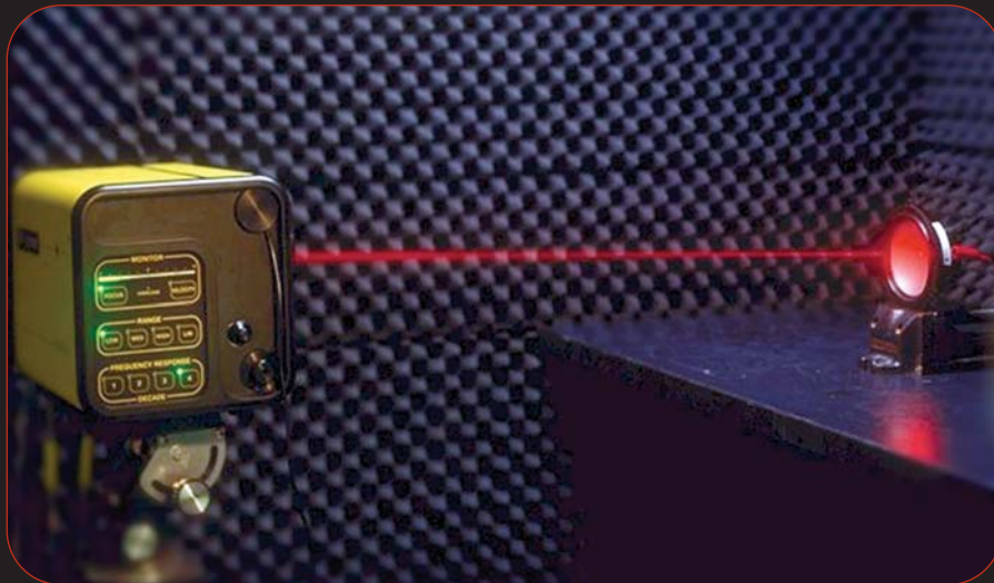
Laser interferometer scanning a transducer diaphragm
