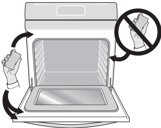
Figure 17: Clean around the door gasket
