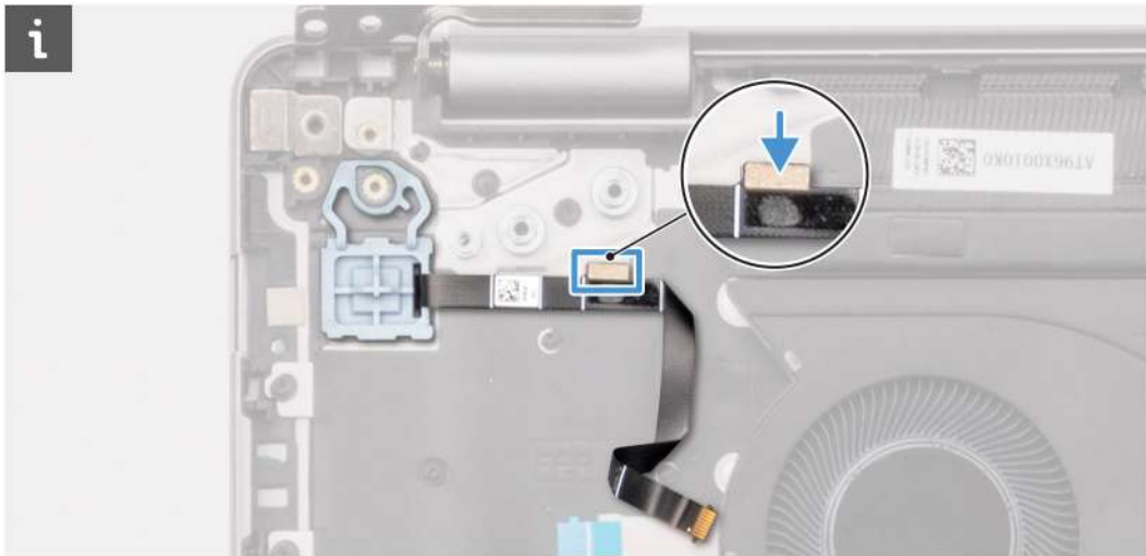
Figure 31. Installing the power button - Grounding tape adhered to keyboard plate
