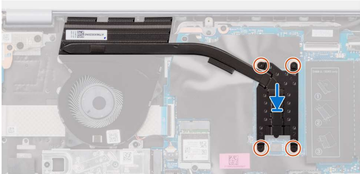
Figure 18. Installing the heat sink
