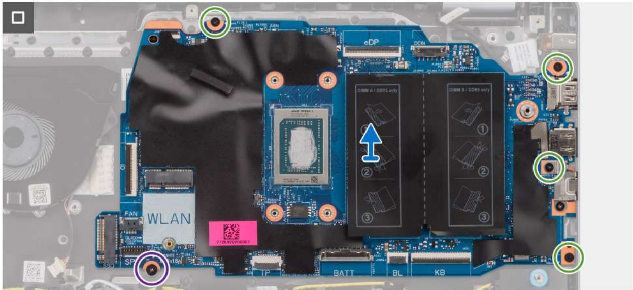
Figure 35. Removing the system board
