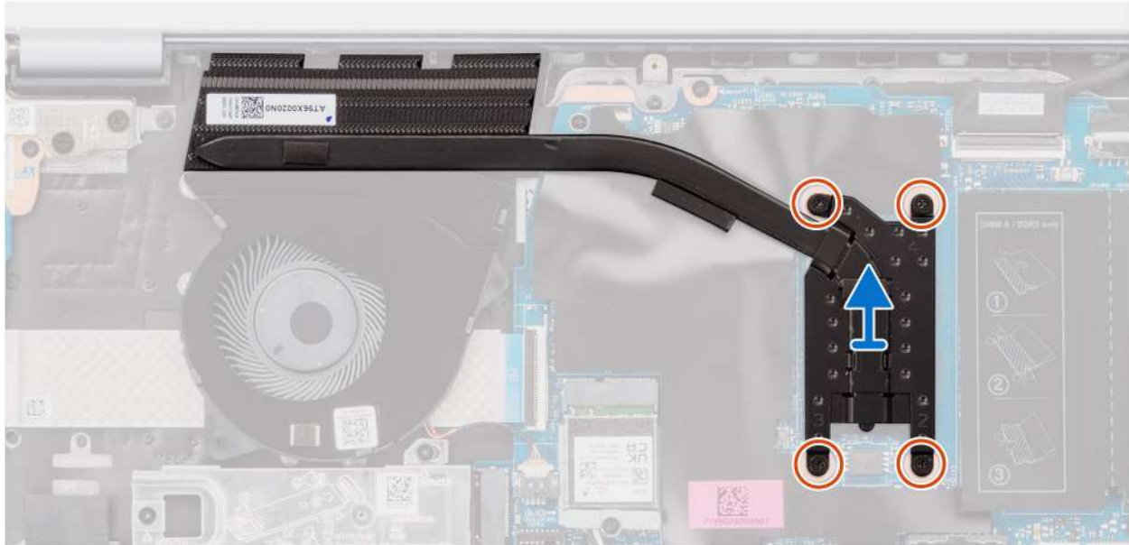
Figure 17. Removing the heat sink
