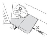
4 Position the middle hinge pin in place to hold the door and insert the two hinge bolts.
