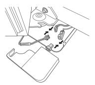
3 Position the bottom hinge cover in its placeand tighten the cover screw 2.
