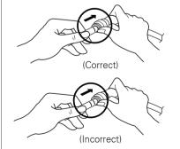
2) Pull the tube to make sure that the tube is tightly fastened.
