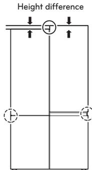
Open the fridge door and use a wrench to rotate the door hinge bolt as shown.
