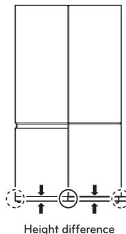
Open the freezer door and use a wrench to rotate the door hinge bolt as shown.
