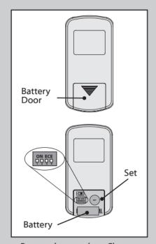
Remove battery door. Change the dip switch settings if the frequency matches a previously installed remote transmitter. Install A23 or MN21 alkaline battery in the proper polarity and replace the battery door. To pair the remote, hold down the Set button for 5 seconds. Pairing is complete when LED button flashes twice.
