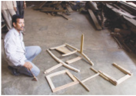
Solid mango components of a dining chair
