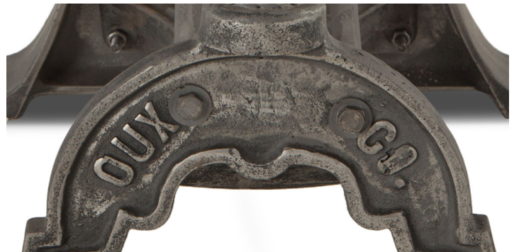
Pits From Casting
