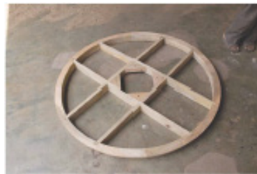
All crossbeams and pedestal hole are fitted together.
