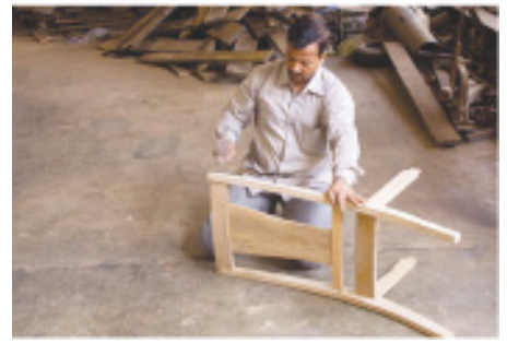
Joints properly aligned and tapped into place.
