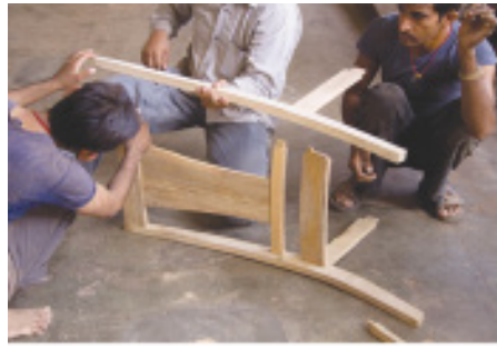
The back is assembled first with mortise and tenon joinery.
