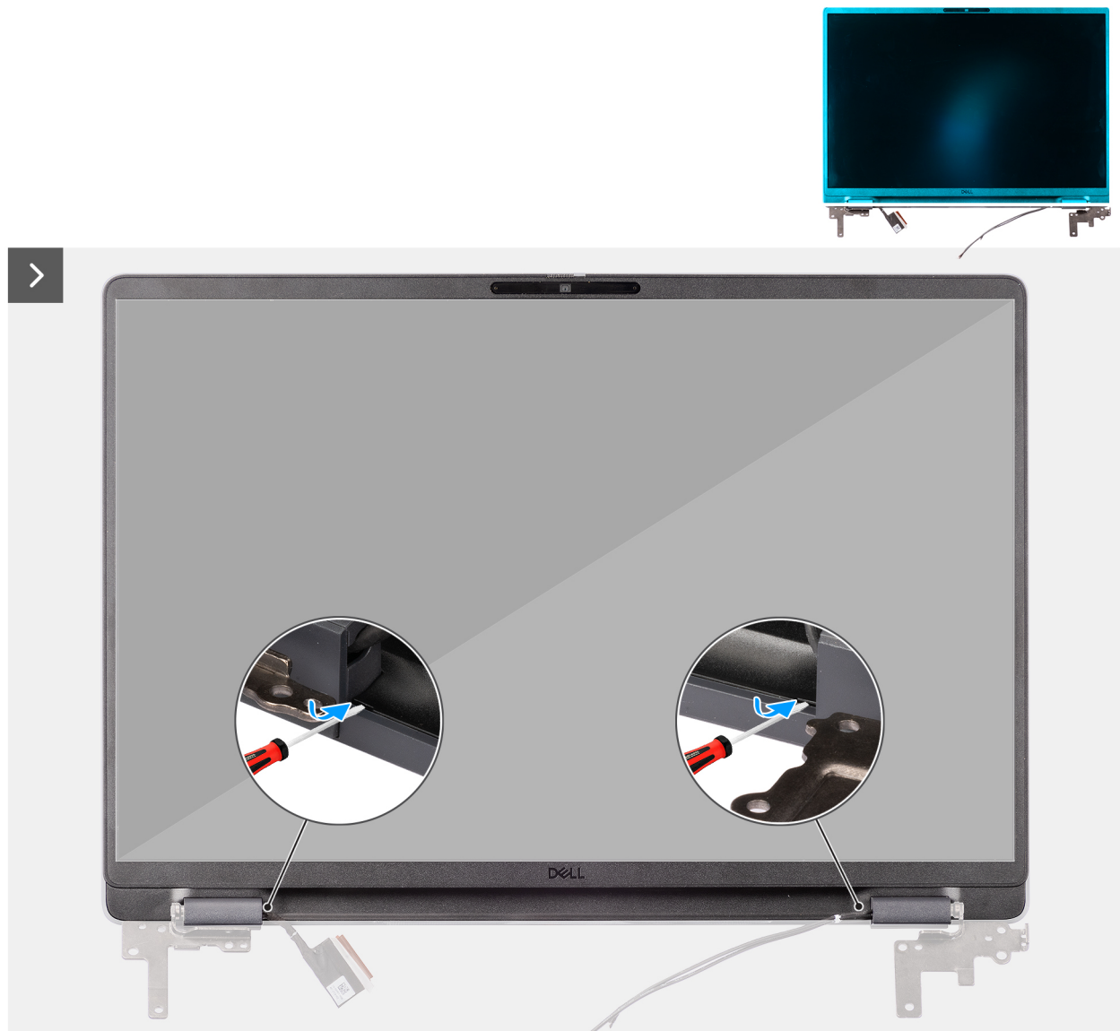
Figure 98. Removing the display bezel
