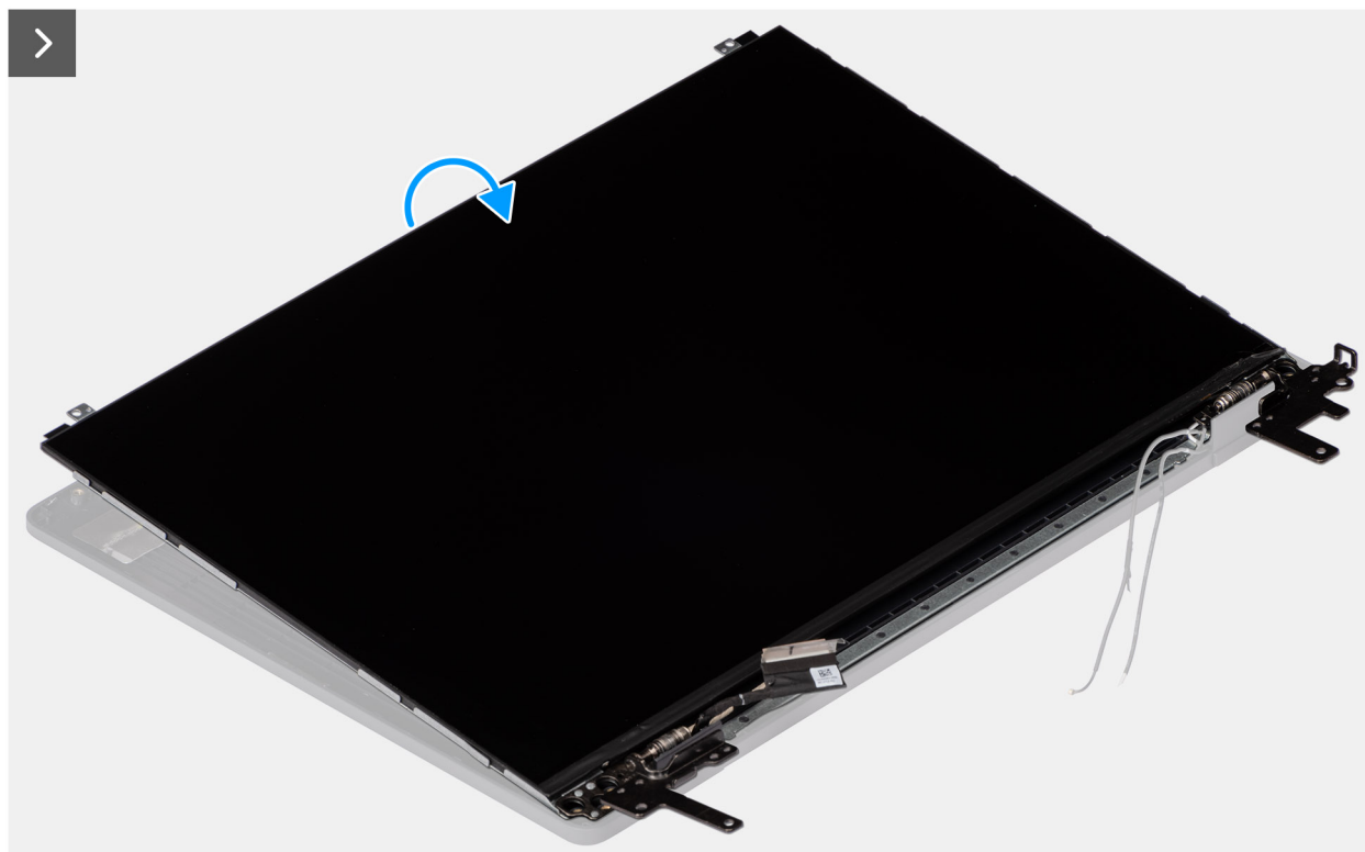
Figure 106. Removing the display-panel assembly
