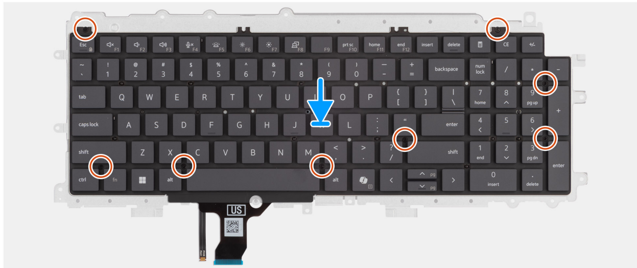
Figure 88. Installing the keyboard support plate
