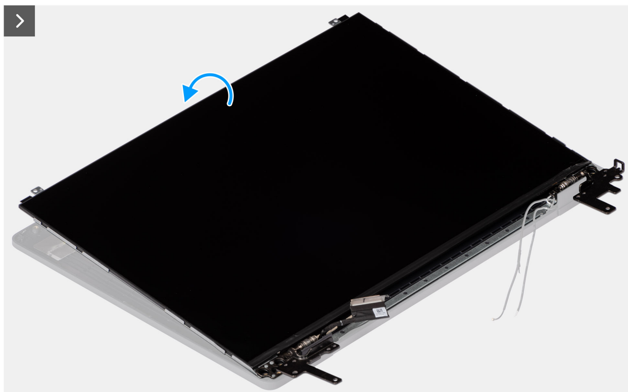
Figure 111. Installing the display-panel assembly
