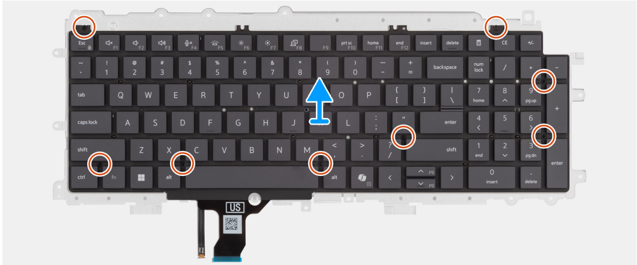
Figure 85. Removing the keyboard support plate
