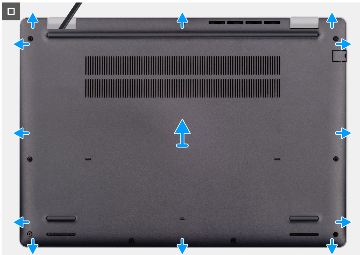
Figure 12. Removing the base cover
