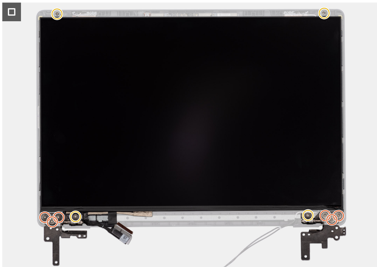
Figure 112. Installing the display-panel assembly
