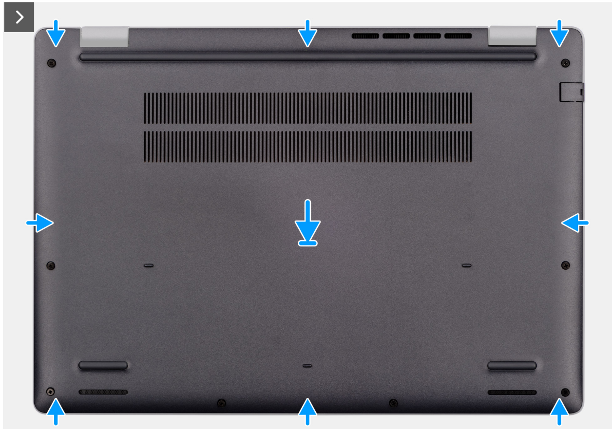
Figure 15. Installing the base cover
