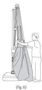
Unfold new replacement canopy. Gather bottom of canopy (larger opening) to the top of canopy (smaller opening).
