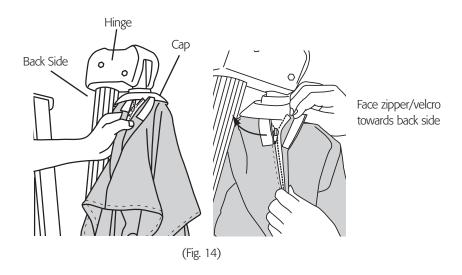
Safely climb down ladder. Line up ends of canopy with spring loaded rib ends.
