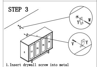
bracket and into drywall anchor.
