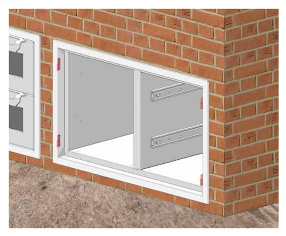
4. Reinstall the drawer(s) by aligning the slides on either side and push the drawer back into the opening. You will hear the release levers click. Open and close the drawer a few times to check for proper function and alignment. There are adjustment screws on either side of the drawer should vertical adjustment be needed. Reinstall the door back on the pins - there is no adjustment.
