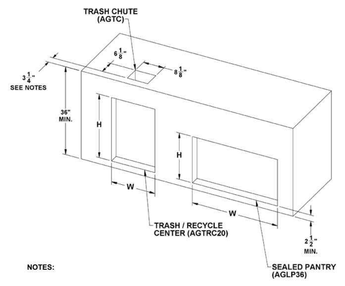
3-1/4" DIMENSION FOR TRASH CHUTE IS MEASURED FROM FACE OF ISLAND STRUCTURE AND DOES NOT INCLUDE ANY OVERHANG FROM A COUNTERTOP.
