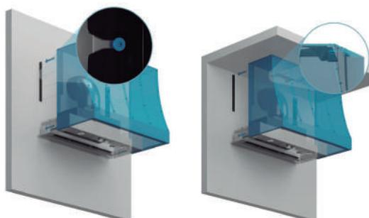
**6** Secure the insert hood to the Shell from the inside placing the screws on the corresponding drill holes.
