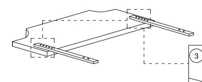
Secure each support stand by using 2x JCBB Bolt [1] and 2x M8 Flat Washer [2].
