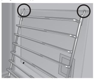
Push upward the rack support as shown below.
