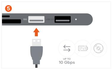
Connect one USB 3.0 Type-A device for high speed data transfer up to 10 Gbps.
