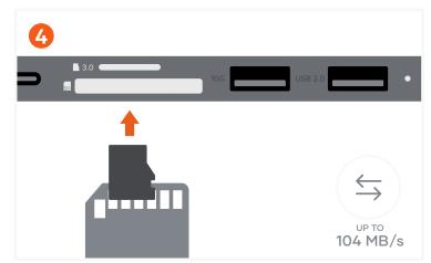
Insert micro/SD cards into adapter's card reader slots. Cards can be read simultaneously.
