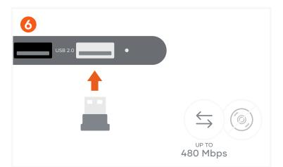
Connect one USB 2.0 Type-A device for low-power devices up to 480 Mbps. Recommended for USB-A peripherals or wireless receivers.
