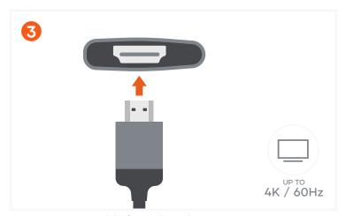
Connect HDMI cable from the adapter to a 4K HDMI-equipped display.
