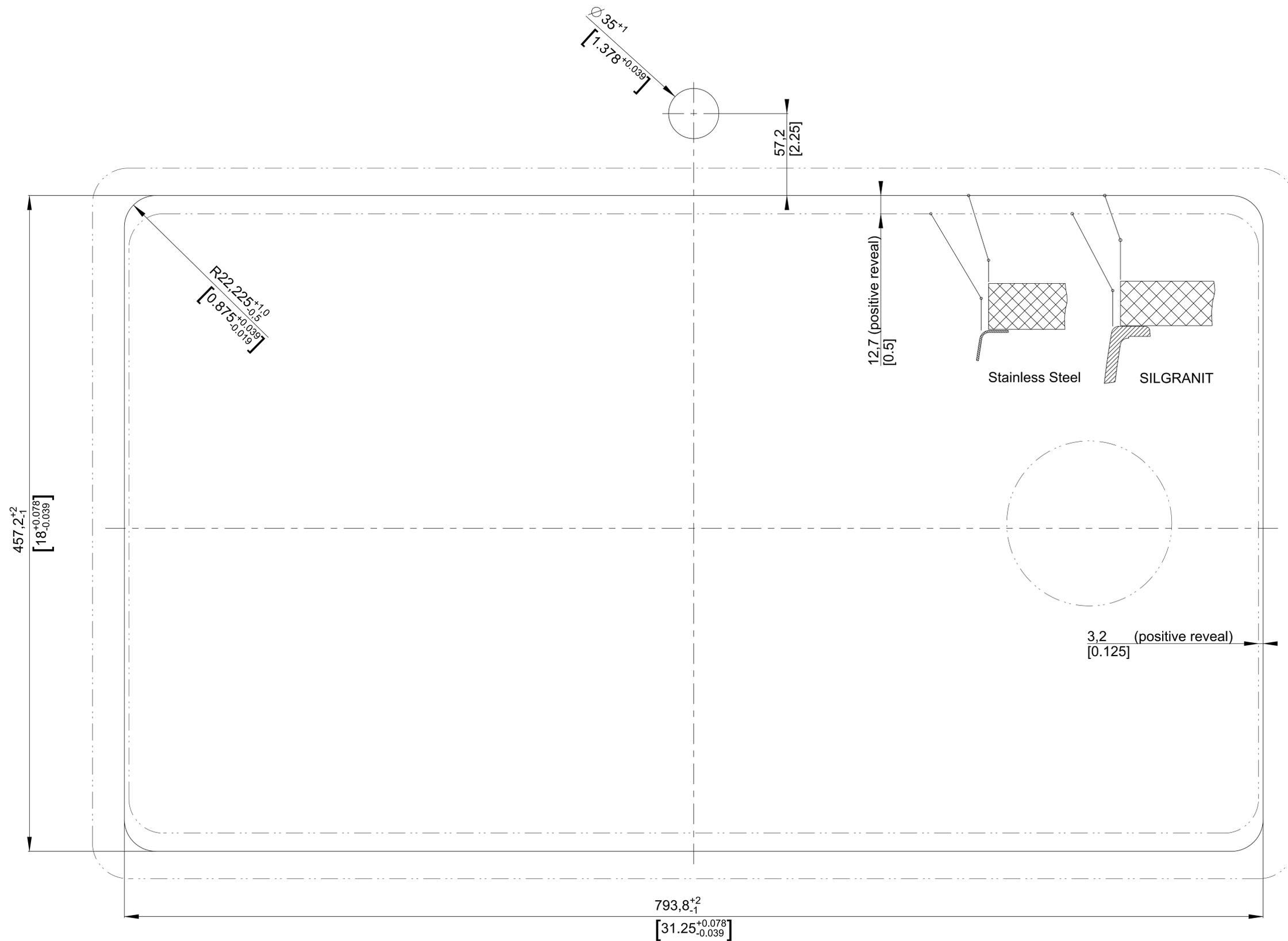
For cut-out geometry please use only dxf-layer "cut-out"
