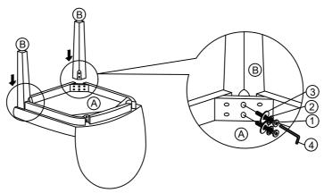
STEP 2: Assemble Back leg (C) to Seat (A) using Allen key (4) with hardware 1, 2, and 3.
