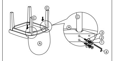
STEP 3: To level the chair, stand the chair up on a flat surface and tighten all the screws using Allen key (4).
