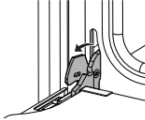
Oven door hinge lock in unlocked position
