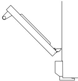
Holding the door on both sides, lift door back up to 45° and carefully pull the door out and away from the hinges.
