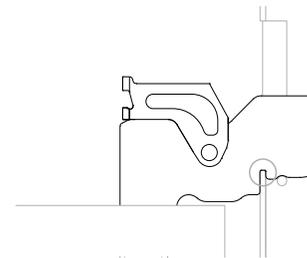
Open the door completely and ensure both hinges are secured by the correct notches.
