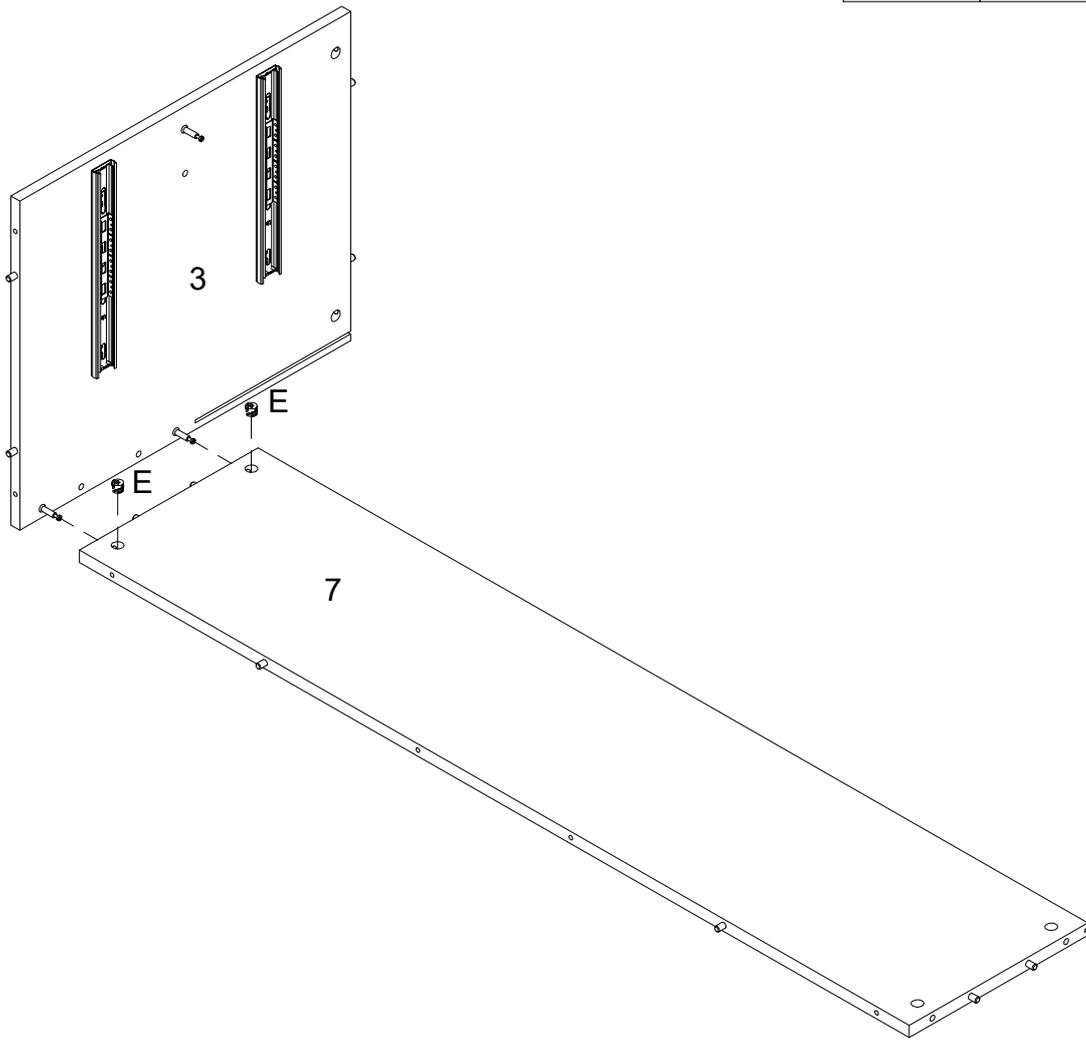
Using Cam lock(E) secure part (3) to part (7) with Philips head screwdriver as per diagram.
