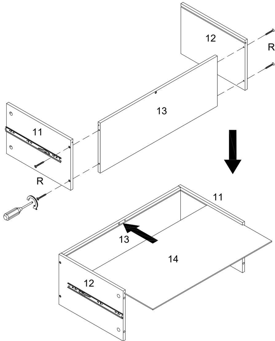
Using screw (R) attach parts (11,12) to part (13) with Philips head screwdriver ,then put part (14) as per diagram.
