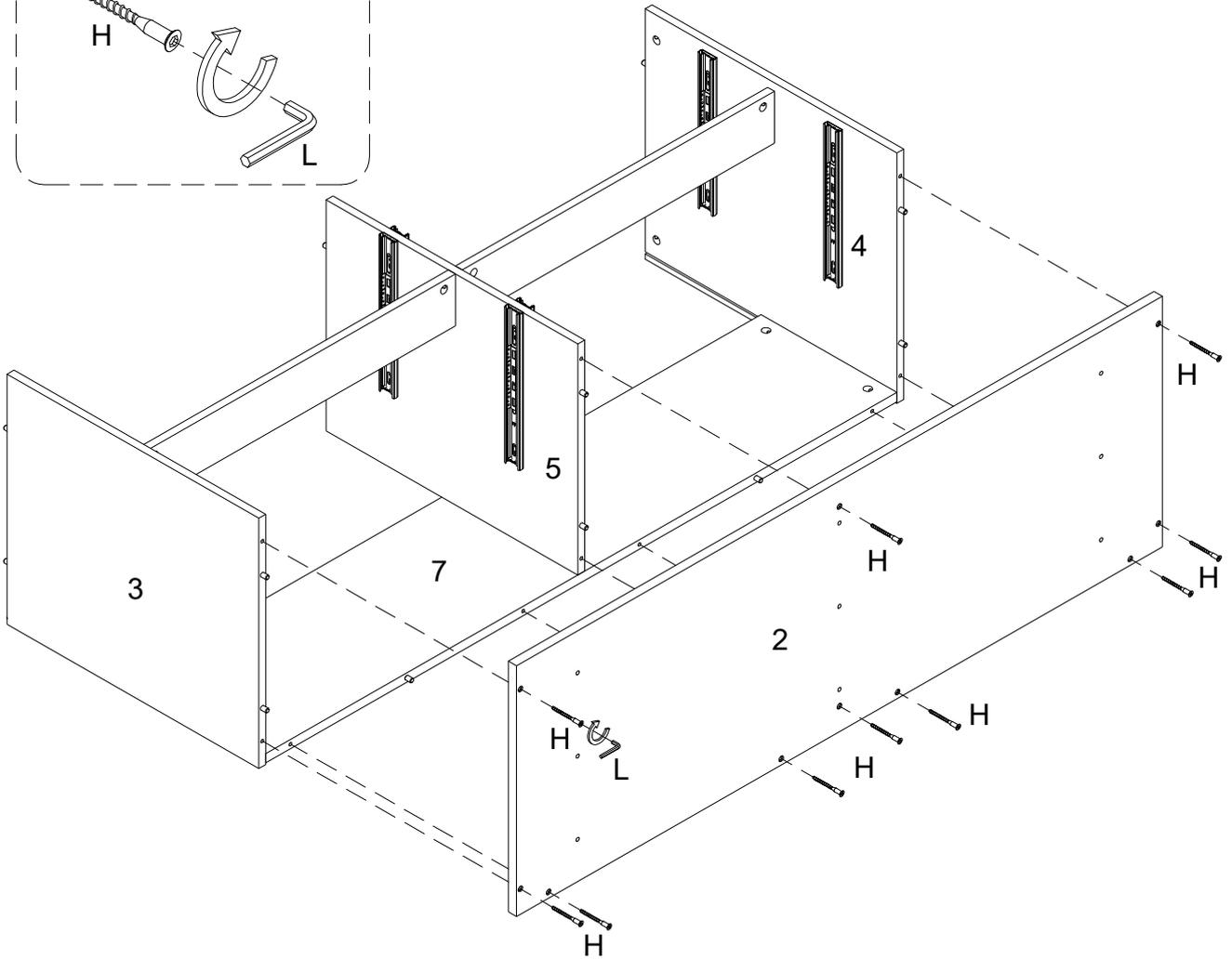
Using screw (H) attach part (2) into parts (3,4,5,7) with Hex key (L) as per diagram.
