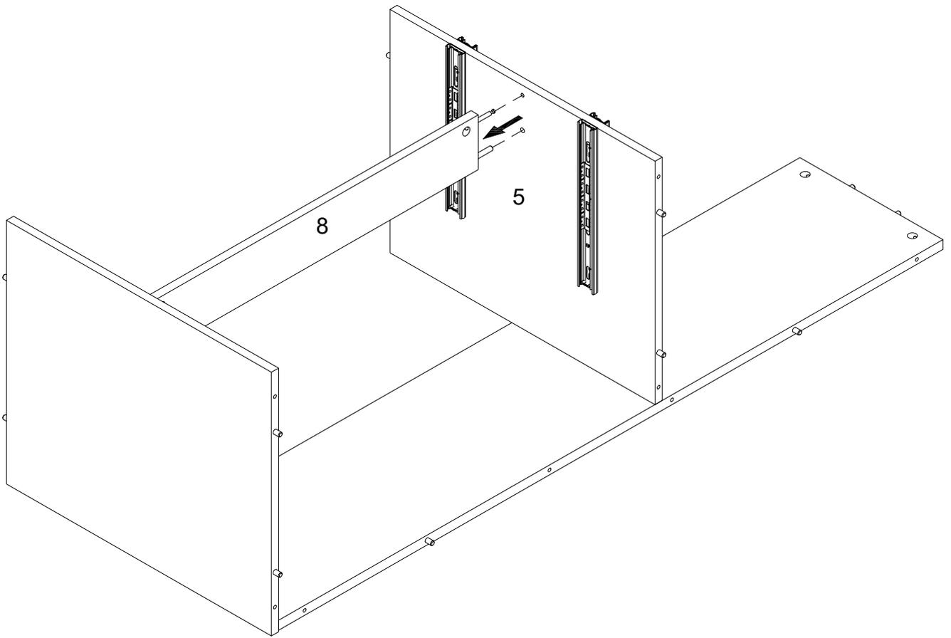
Attach part (5) into part (8) as per diagram.
