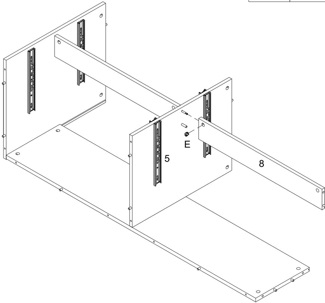
Using Cam lock(E) secure part (8) to part (5) with Philips head screwdriver as per diagram.
