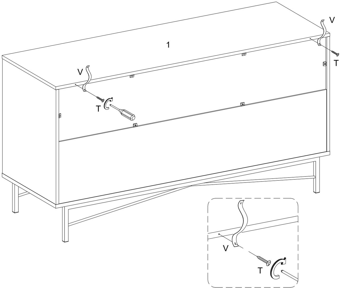
Using screw (T) attach plastic strap (V) into part (1) with Philips head screwdriver as per diagram.
