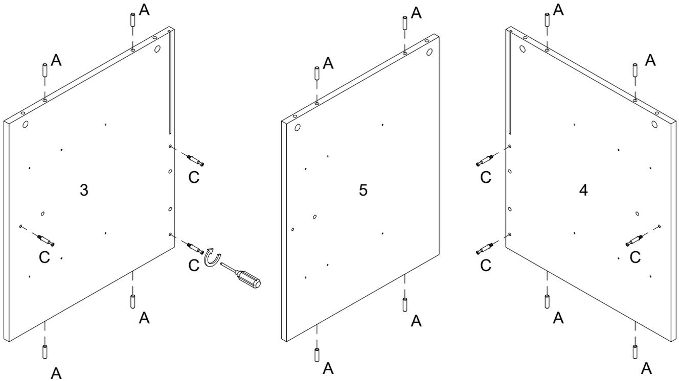
Insert wooden dowel (A) into parts (3,4,5) , then secure cam bolt (C) into parts (3,4) with Philips head screwdriver as per diagram.
