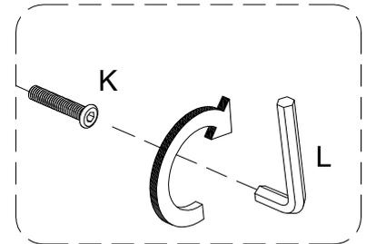
Using bolt (K) attach part (10) to part (2) with Hex key (L) as per diagram.
