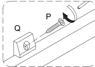
Using screw (P) secure plastic wedge (Q) to part (6) with Philips head screwdriver as per diagram.
