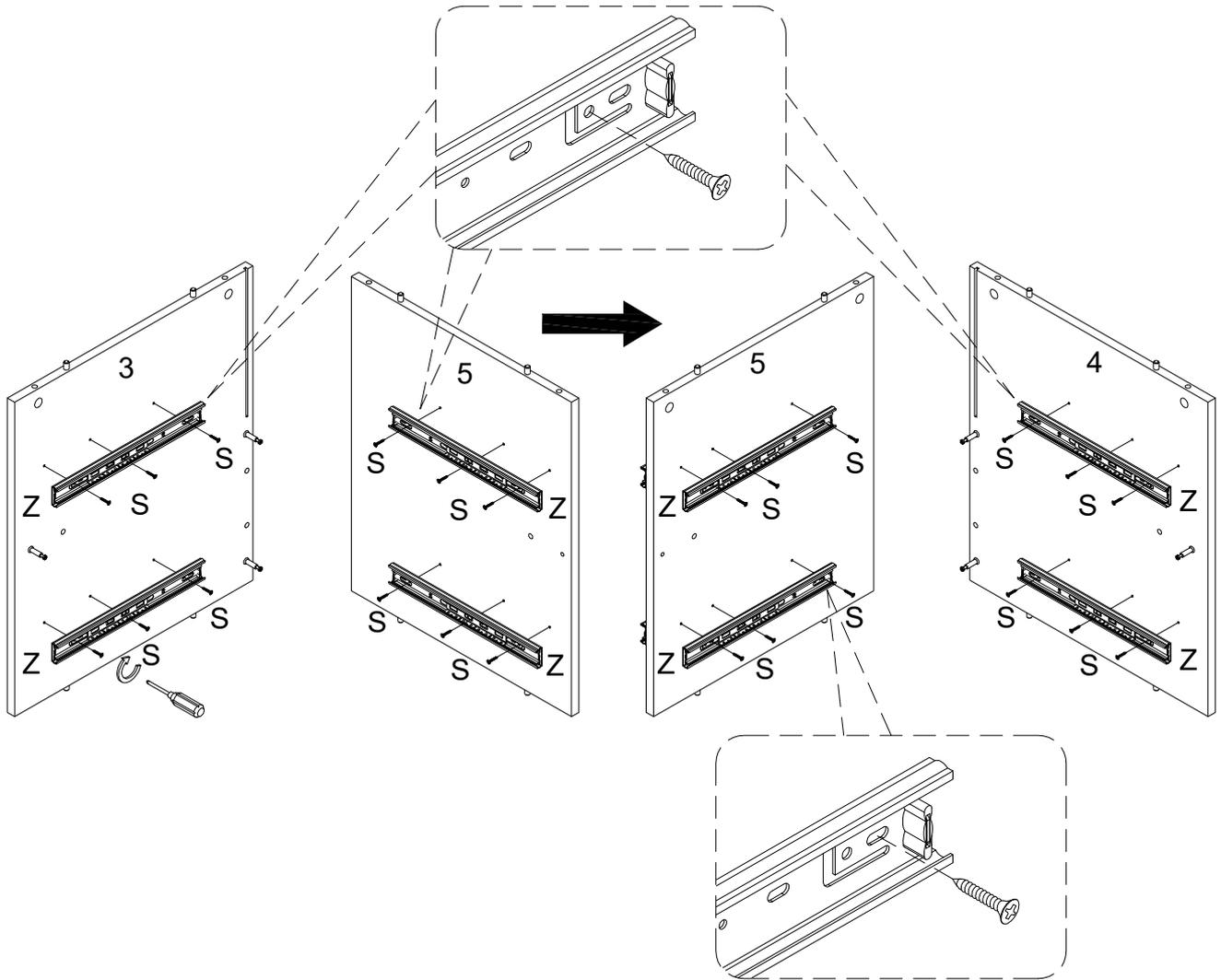
Using screw (S) attach drawer slider (Z) into parts (3,4,5) with Philips head screwdriver as per diagram.
