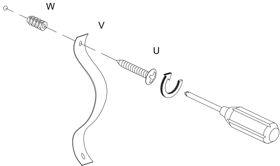
Using screw (U) attach plastic strap (V) into Nut (W) to wall with Philips head screwdriver as per diagram.
