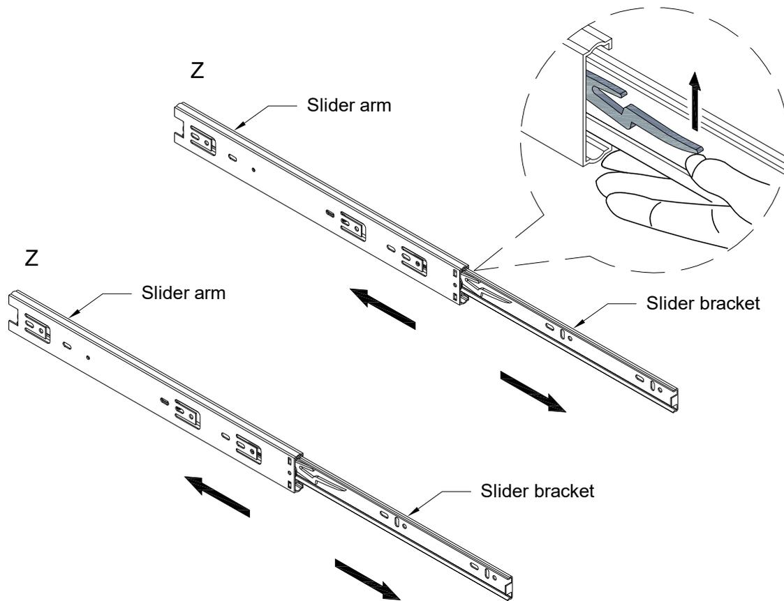
Pick up the slider arm (Z) and separate the slide runner for the following Steps. Extend the slide runner all the way forward, press the plastic release lever of the slider arm up and pull the slide runner complete out .
