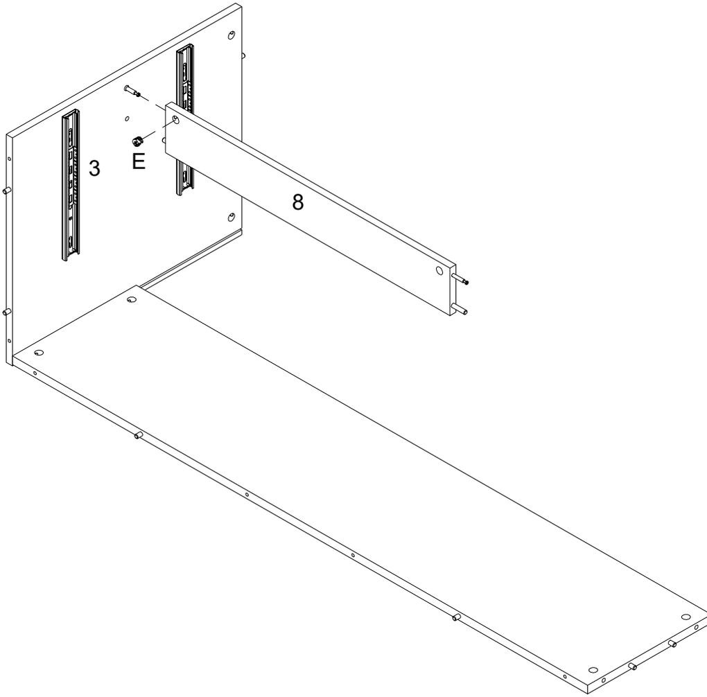
Using Cam lock(E) secure part (8) to part (3) with Philips head screwdriver as per diagram.
