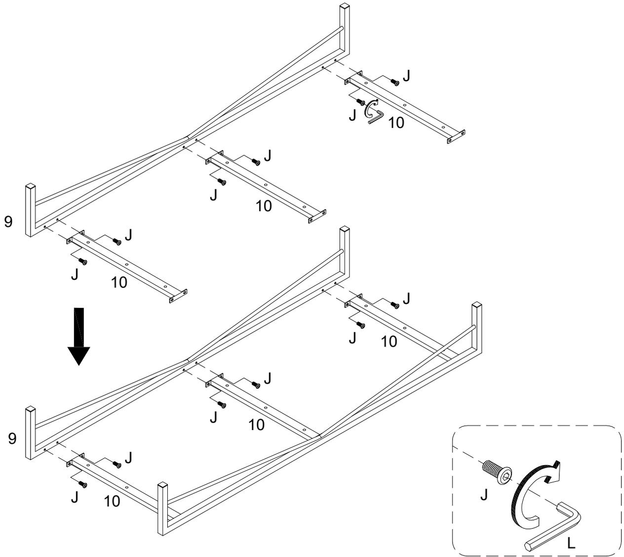
Using bolt (J) attach part (10) to parts (9) with Hex key (L) as per diagram.
