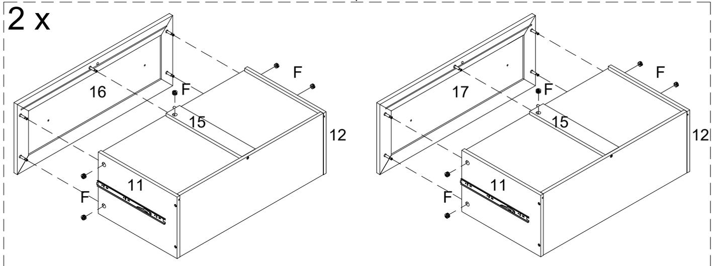
Using screw (R) attach part (15) to part (13) with Philips head screwdriver ,then using cam lock (F) secure parts (16,17) to parts (11,12) with Philips head screwdriver as per diagram.
