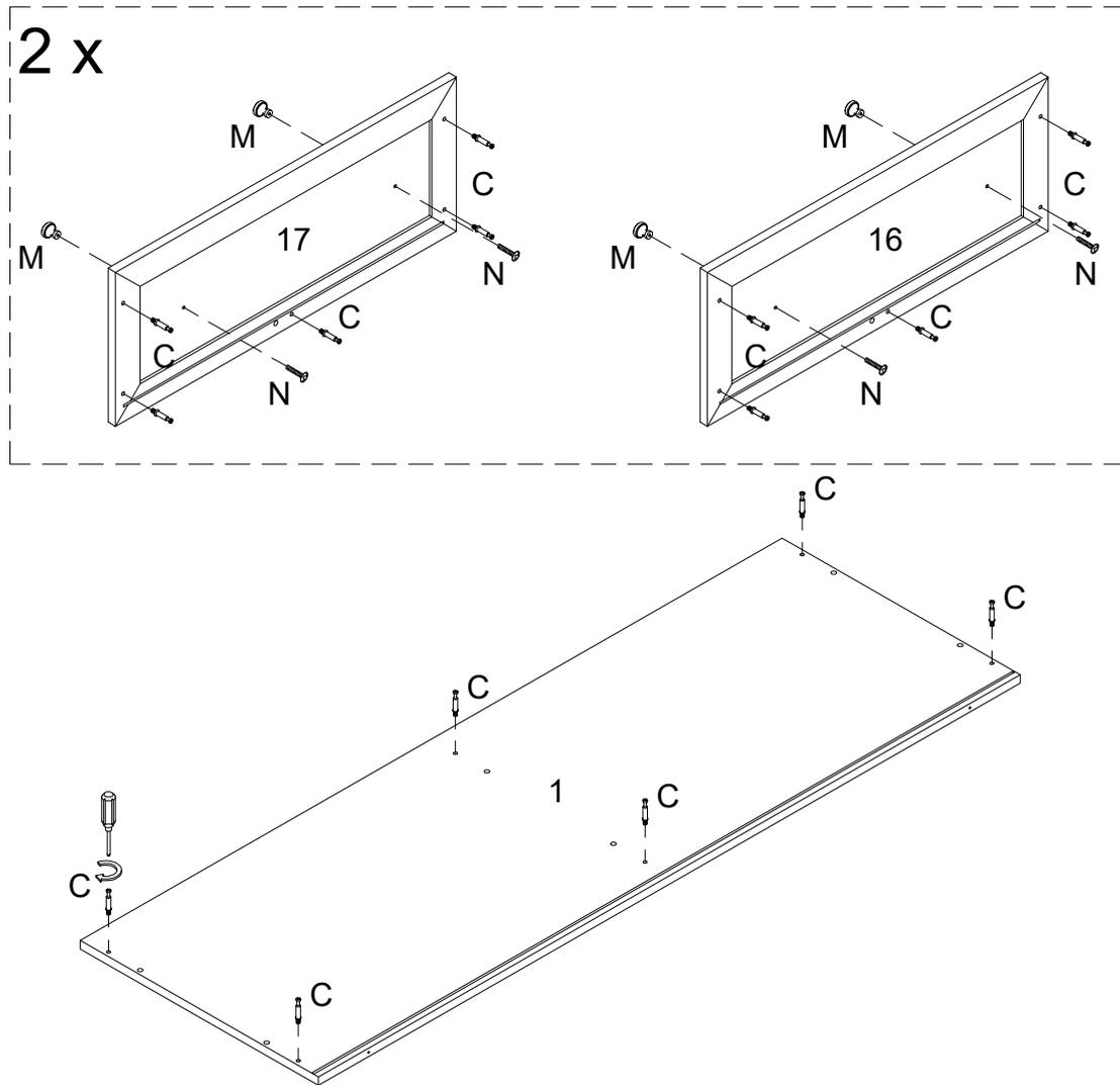
Secure cam bolt (C) into parts (1,16,17) ,then using handle bolt (N) secure handle (M) into parts (16,17)with Philips head screwdriver as per diagram.
