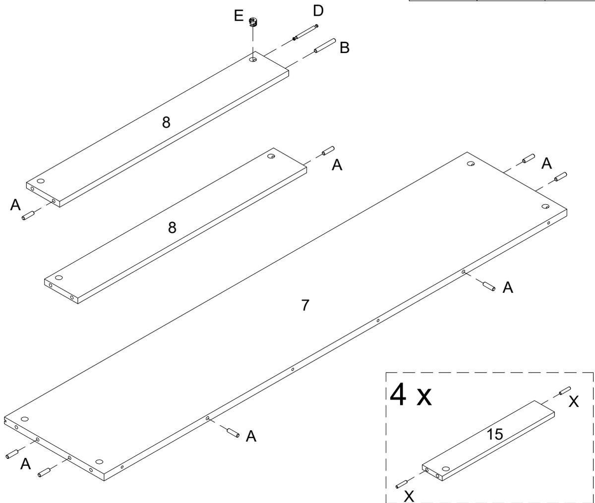
Insert wooden dowel (A) into parts (7,8) and wooden dowel (B) into part (8), wooden dowel (X) into part (15) , then using cam lock (E) secure cam bolt (D) into part (8) with Philips head screwdriver as per diagram.
