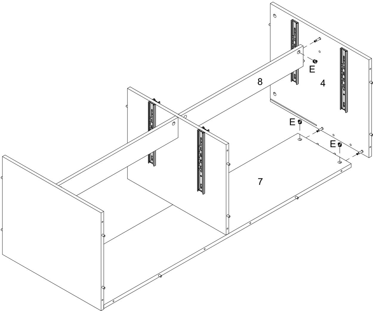
Using Cam lock(E) secure part (4) to parts (7,8) with Philips head screwdriver as per diagram.
