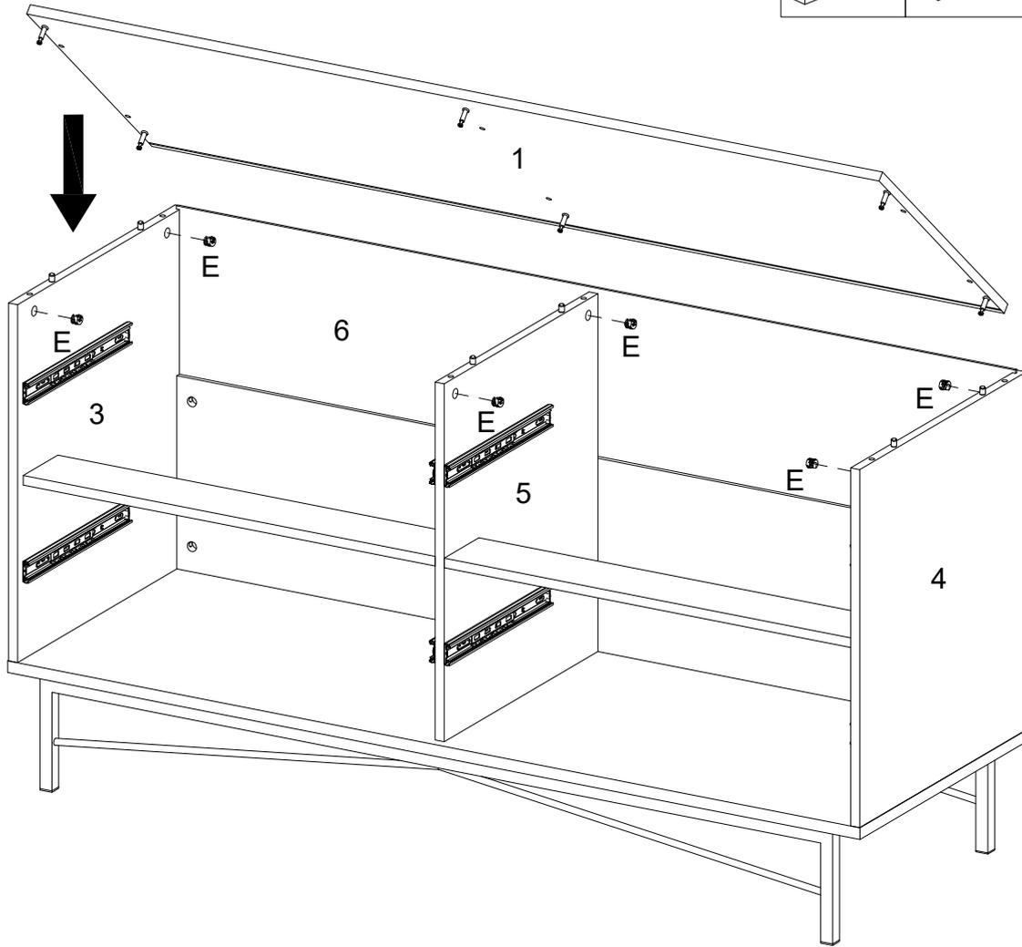
Using cam lock (E) secure part (1) into parts (3,4,5) with Philips head screwdriver as per diagram.
