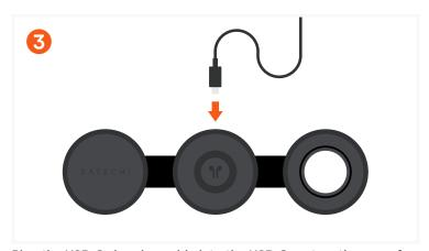
Plug the USB-C charging cable into the USB-C port on the rear of the charger. The front LED indicator will briefly turn on, turn off, then flash once to indicate that the charger is connected to power.
