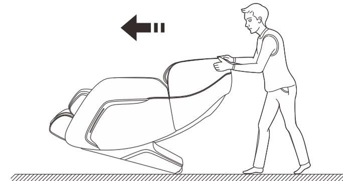
Note: Before movement you must turn off the power first and then unplug the power cord, as well as the controller cord.
