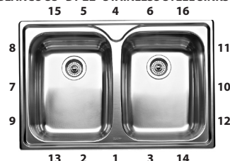
PROPER TORQUE SEQUENCE CHART FOR BLANCO 33" BY 22" STAINLESS STEEL SINKS
