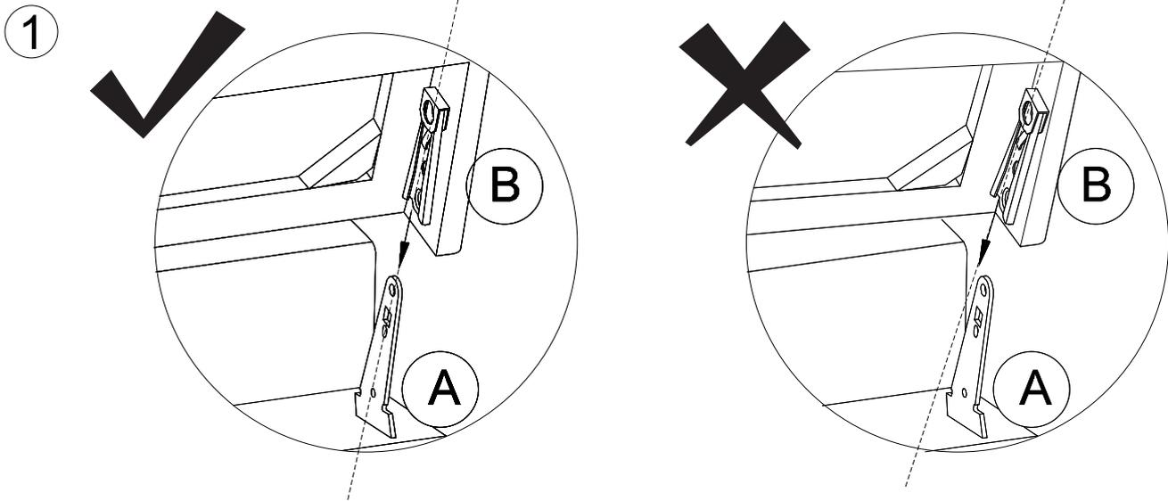
Make sure to align the two receiver clips on each side of the recliner back (B) with the two support (A) arms in the chair base to the center line.
