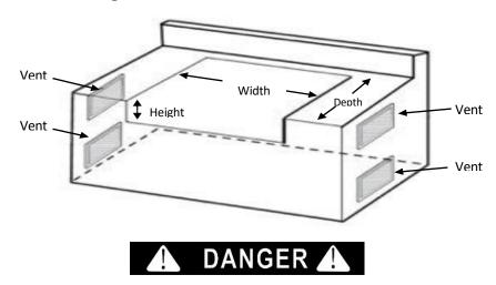
Minimum of 2 vents, but optimally 4 vents, per cabinet that has any sort of gas supply or connection. Each vent must be at least 20 sq in in size and have access to outside/fresh air.
