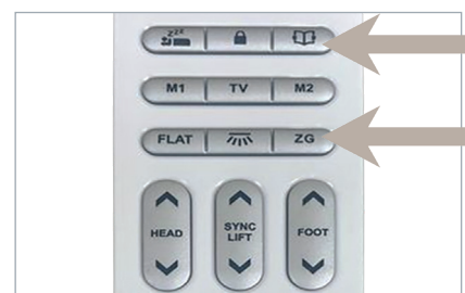
Method 2: Press the Reading + ZG buttons to reset the system.
