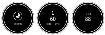
Rotate the knob to MEMORY interface, press the knob once to enter. Rotate the knob to select one position. Press the knob again, and the seat will move to the preset position.
