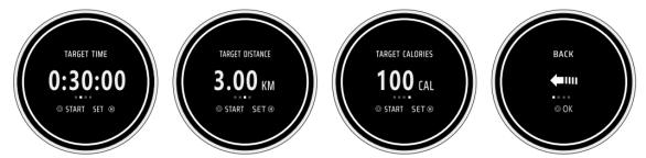
Press the knob and hold to enter SET interface. Turn the knob to adjust parameters accordingly. Press the knob once to start.
