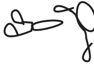
Wire clip (2) (for securing Drain hose joiner)
