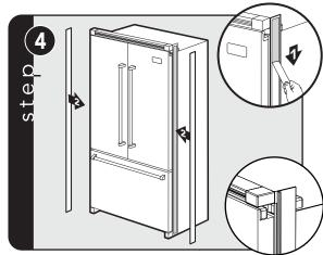
Remove adhesive backing for the side trim. Locate the top of the side trim with the top of the grille assembly. Press the side trim into the refrigerator cabinet at the center location.
