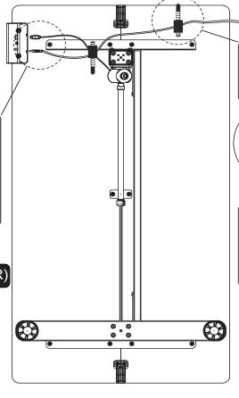
THEN: Attach the cable clips F and secure the cables as shown.
