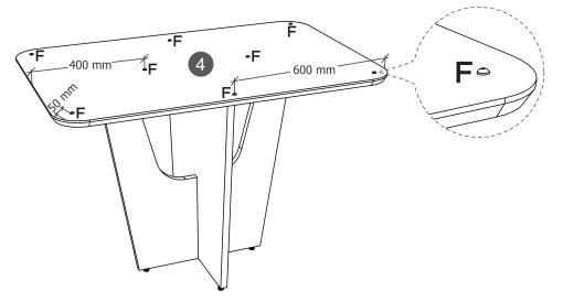
THEN: Carefully place the glass top #5 over the silicone bumpers aligning with the tabletop #4.
