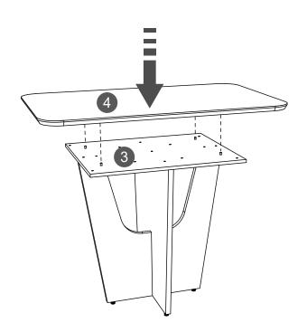
THEN: Secure the wood tabletop #4 to panel #3 with screws B from underneath
