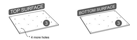
THEN: Attach to the TOP surface of panel #3 the wooden dowels C on the indicated holes.
