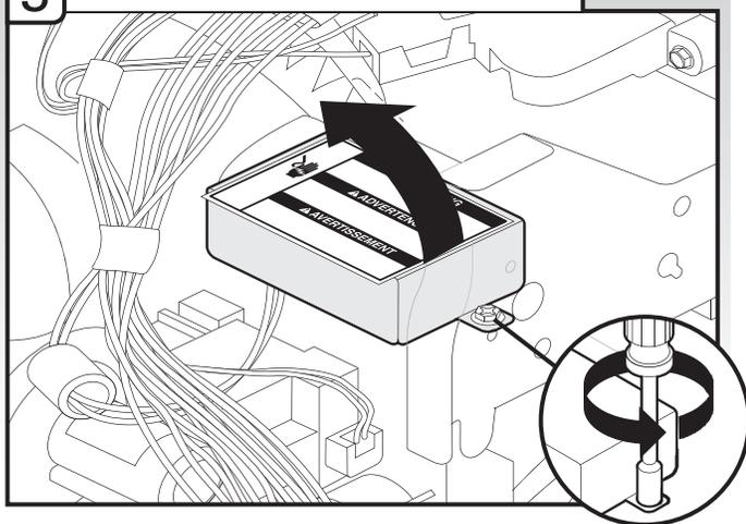
Using a  $\frac{1}{4}$ " hex head socket, nut driver or Torx® T20® screwdriver, remove terminal box cover. Retain for later use.
