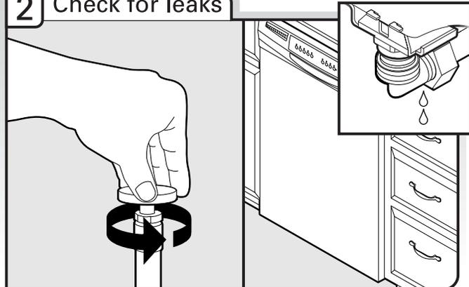
Place paper towel under 90° elbow fitting. Turn on water supply and check for leaks. If leak occurs, repeat previous step.
