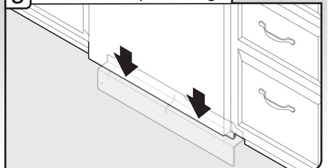
Check that the lower edge of the lower panel contacts the floor. Adjust if necessary.
