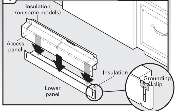
Check that grounding clip is attached to the lower panel. Position the lower panel behind the access panel. On some models there is insulation on the access panel that must fall behind the insulation on the lower panel.
