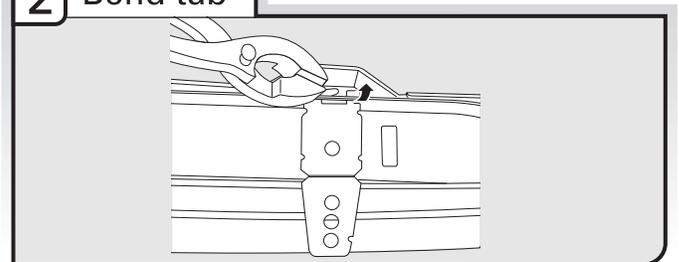
Using a pair of pliers, bend the tab down to secure the bracket in place. Repeat this step for the other side.
