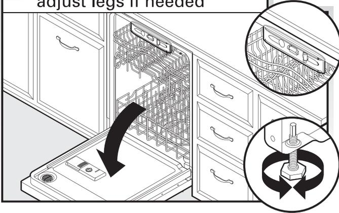
Place level against top front opening of tub. Check that dishwasher is level from side-to-side. If dishwasher is not level, adjust front legs up or down until dishwasher is level.
