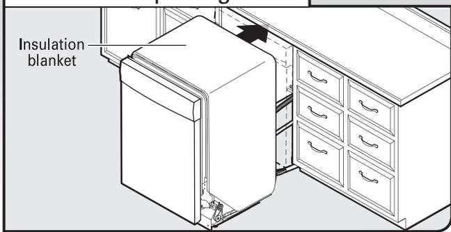
**IMPORTANT:** If wheels were removed, cover the floor when moving the dishwasher to avoid damage to the floor. Slowly move dishwasher completely into cabinet opening. Do not kink or pinch water line, drain hose, power supply cord or direct wire between dishwasher and cabinet. Remove cardboard from under dishwasher.
