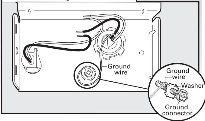
Remove the green grounding screw and place through the ring terminal of the green ground wire. Reattach and tighten the green screw.
