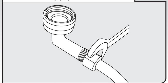
Connect the  $\frac{3}{8}$ " compression fitting to the water supply line prior to installing the unit into the cabinet opening. Attach such that the  $\frac{3}{4}$ " connection is facing upward as shown above.
