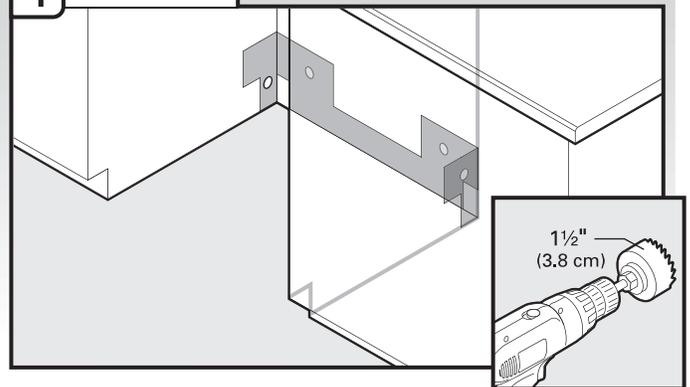
If needed, drill a 1 1/2" (3.8 cm) diameter hole in cabinet wall or side of the opening closest to the sink.
