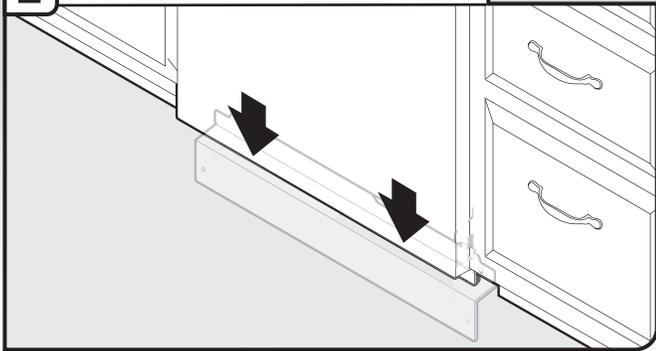
Check that the lower edge of the access panel touches the floor. Adjust if necessary.
