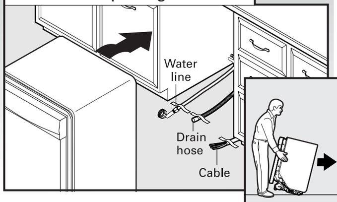
**IMPORTANT:** Double-check correct placement of utilities. Grasp the sides of the dishwasher at the edges of the door panel. Tilt dishwasher backward on wheels and move dishwasher close to cabinet opening.
