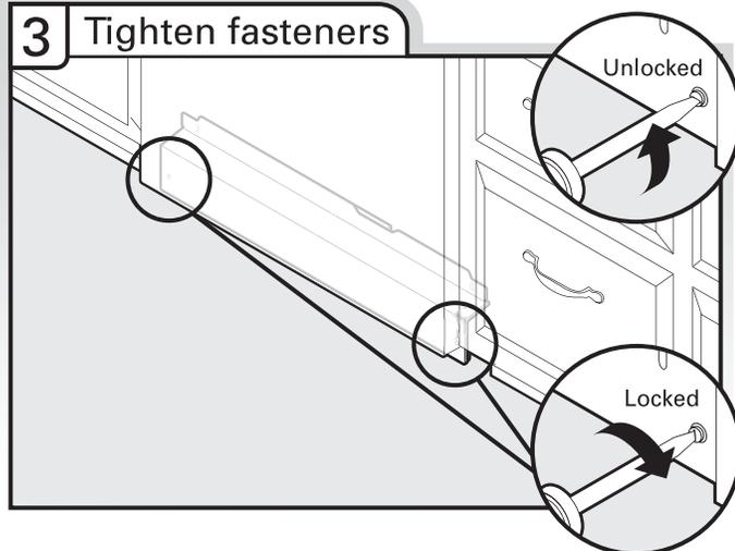
Using a flat-blade screwdriver, turn the fasteners 1/4 turn clockwise to lock into place. The fasteners slot will be straight up and down when properly locked.
