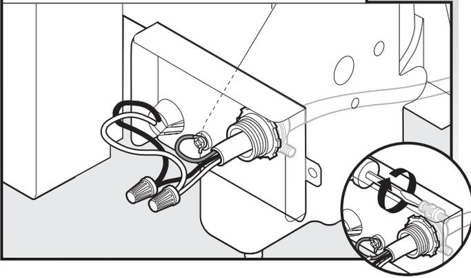
Tighten strain relief screws to secure cable.
