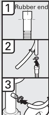
1. Connect rubber end of drain hose to air gap and cut if needed.
