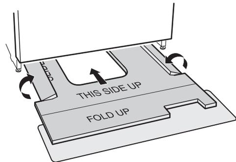
4. Fold the front end of the pad up into position. Make sure the vinyl pad is tucked up behind the door and the dishwasher front legs, as shown.
