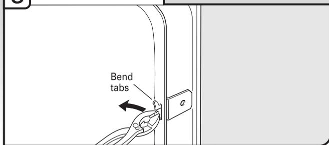
Push bracket into slot on the side of dishwasher, and bend tab in toward the side of the dishwasher so that it keeps the bracket in place. Repeat this step for the other side of the dishwasher.
