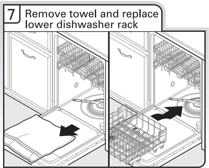
Remove towel from dishwasher. Reinstall the lower dish rack. If needed, see website for animated representation of this step. Visit [www.jenn-air.com/anchoring](http://www.jenn-air.com/anchoring) under FAQ tab.
