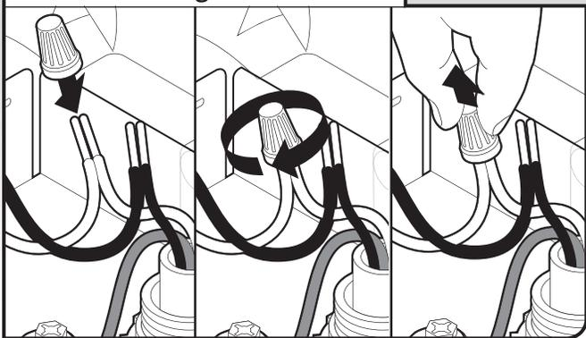
**NOTE:** Do not pre-twist stranded wire. Twist on wire connector. Gently tug on wires to be sure both are secured.
