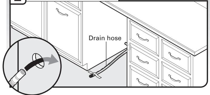
Route drain hose as shown through hole in cabinet to the front center of opening where drain connection will be made. Tape drain hose to the floor in area shown. This will prohibit it from moving when dishwasher is moved into cabinet opening.
