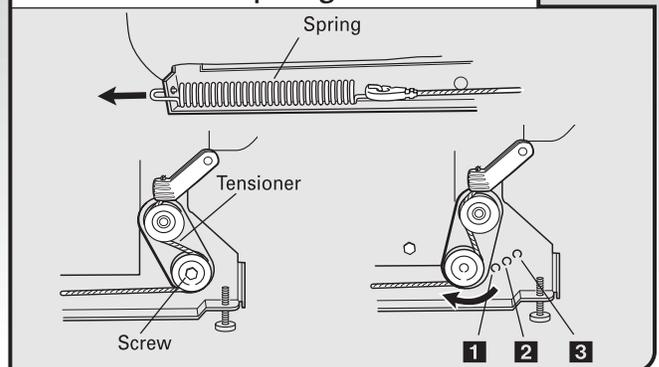
To adjust the door spring tension, unhook the spring from the rear leg of dishwasher.
