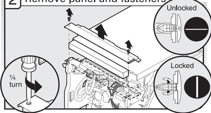
Using a flat-blade screwdriver, turn the plastic fasteners  $\frac{1}{4}$  turn counterclockwise to unlock them. Remove panel. Do not remove tech sheet from access panel.
