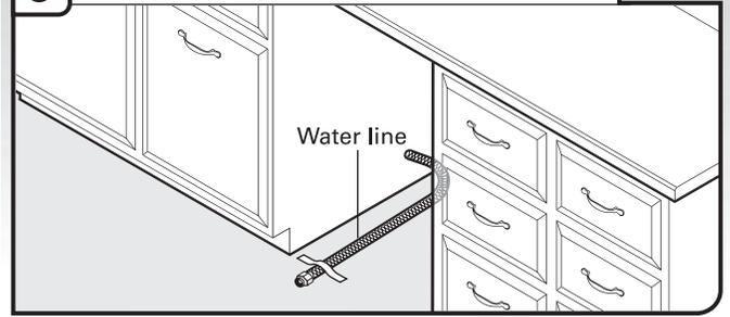
Route water line and tape it to the floor in area shown. This will keep it from moving when dishwasher is moved into cabinet opening.
