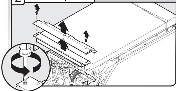
Using a  $\frac{1}{4}$ " hex head socket, nut driver or Phillips screwdriver, remove 2 screws attaching access panel and lower panel to dishwasher. Do not remove tech sheet from access panel.
