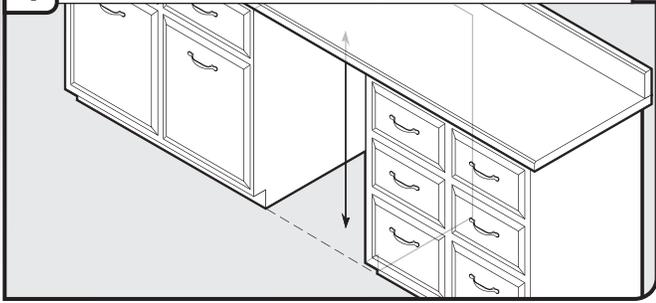
Measure height of cabinet opening from underside of countertop to floor where dishwasher will be installed (you will need to measure the lowest point on the underside of the countertop and the highest point on the floor). Refer to "Dishwasher Height Adjustment Chart" for wheel position and the number of turns needed.
