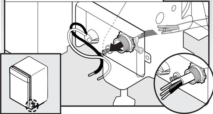
Route cable so that it does not touch dishwasher motor or lower part of dishwasher tub. Pull cable through UL Listed/CSA Approved strain relief in terminal box. Strain relief is not supplied with the dishwasher. Owner must purchase a  $\frac{7}{8}$ " screw-in type strain relief.
