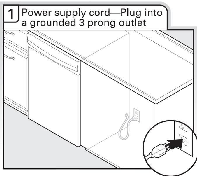
Plug into a grounded 3 prong outlet. Check that power supply cord does not touch dishwasher motor or lower part of dishwasher tub.
