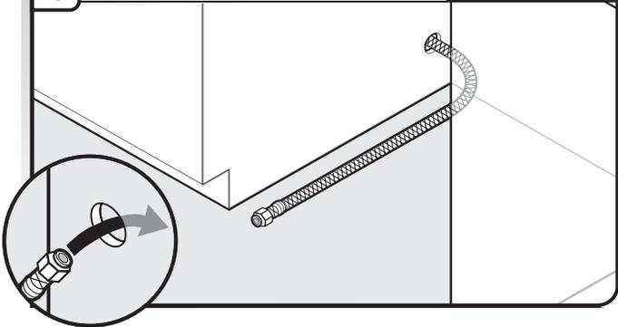
Slowly route water supply line through hole in cabinet. (If you are using copper tubing, it will bend and kink easily, so be gentle.) It should be far enough into the cabinet opening to connect it to the dishwasher inlet on the front left side of the dishwasher.
