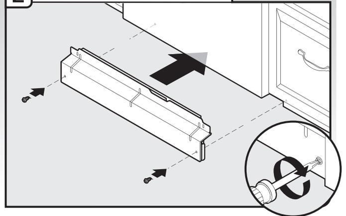
Hold the 2 panels together and place them against dishwasher leg. Using a Phillips or 1/4" screwdriver, reinstall the screws through the holes in the access panel and the slots in the lower panel.
