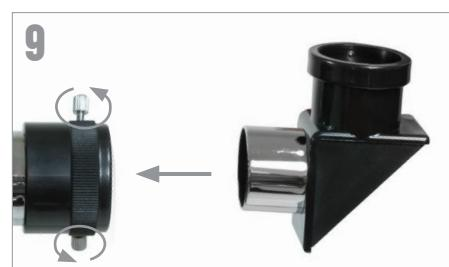
Locate the erect image diagonal and remove the plastic covers. Insert the barrel of the diagonal into the focuser and secure in place by tightening the set screws.
