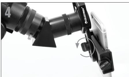
Loosen the knob on the bottom of the adapter that secures the phone clamp to the eyepiece clamp. Slide the phone clamp up and down and rotate it left and right until your camera is looking down through the eyepiece of the telescope. Tighten the knob on the bottom of the adapter to secure it in place.
