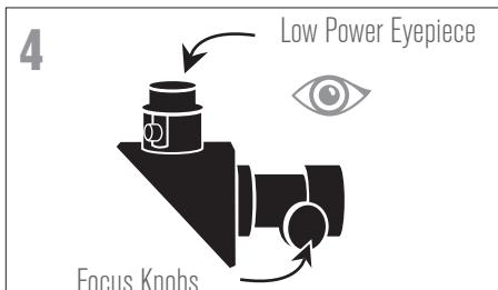
Look through the telescope's 20mm eyepiece. Gently turn the focus knobs to adjust the sharpness of the image.
