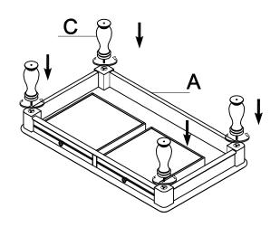
NOTE, WAIT TO TIGHTEN ALL COMPONENTS COMPLETELY UNTIL UNIT IS FULLY ASSEMBLED. THIS WILL ALLOW FOR EASIER ASSEMBLY.
