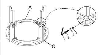
**STEP 2** Attach bottom panel (B) to the legs (C) by using allen key (1), bolts (2) spring washer (3) and flat washer (4).
