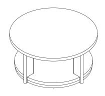
**STEP 1** Attach the legs (C) to the table top (A) by using allen key (1), bolts (2) spring washer (3) and flat washer (4).
