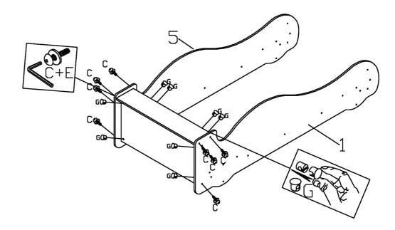
Align side panels (#1,5) to back board, then secure by using bolts (#C) with washers (#E) to barrel nuts (#G). Cover barrel nuts (#G) by using barrel nut caps (#G).
