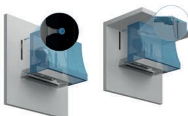
**6** Secure the insert hood to the Shell from the inside placing the screws on the corresponding drill holes.
