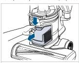
1. Press down on tab to remove Post-Motor Filter cover and pull away from vacuum.
