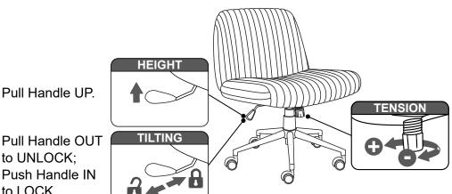
Turn CLOCKWISE for less tension (-); COUTERCLOCKWISE for more tension (+). With less tension, the tilting feels easier.
